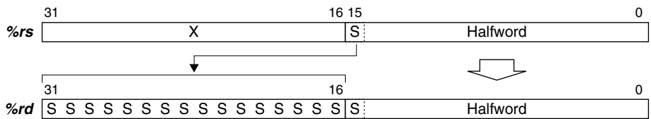
Figure 3.7.1 Signed 16-Bit Transfer (Register → Register)
