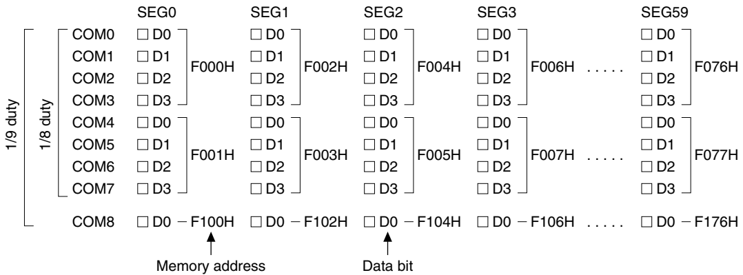
Fig. 4.7.4.1 Correspondence between display memory and LCD dot matrix (S1C63406)
