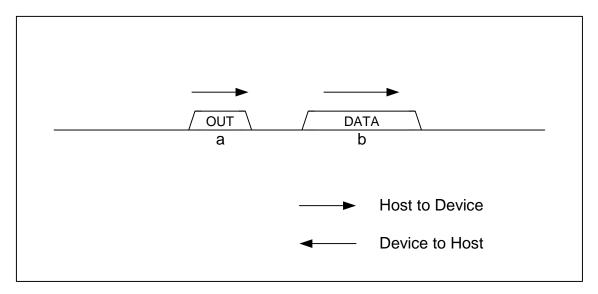
Figure 1-27 Isochronous OUT transaction
