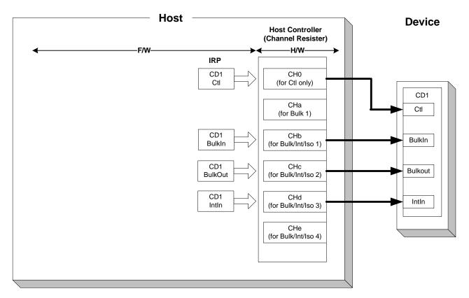
Figure 1-22 Channel usage example (with one communication device connected)
