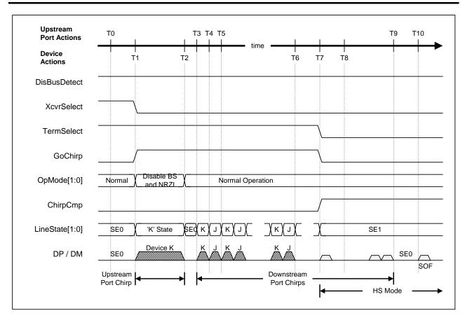
Figure 1-14 HS detection handshake timing (HS mode)
