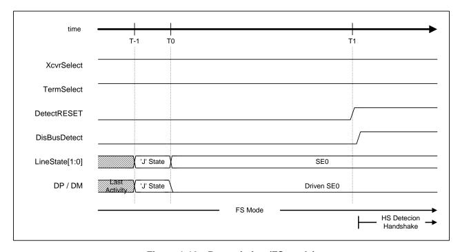
Figure 1-12 Reset timing (FS mode)
