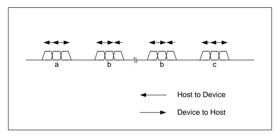
Figure 1-7 Control transfer when data stage is IN
