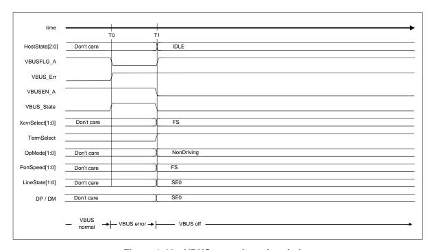
Figure 1-40 VBUS error detection timing
