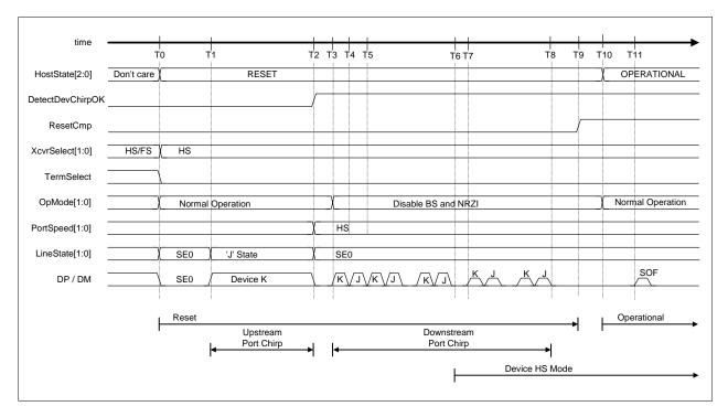
Figure 1-54 Reset timing (HS mode)
