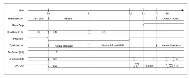
Figure 1-58 Reset timing (LS mode)
