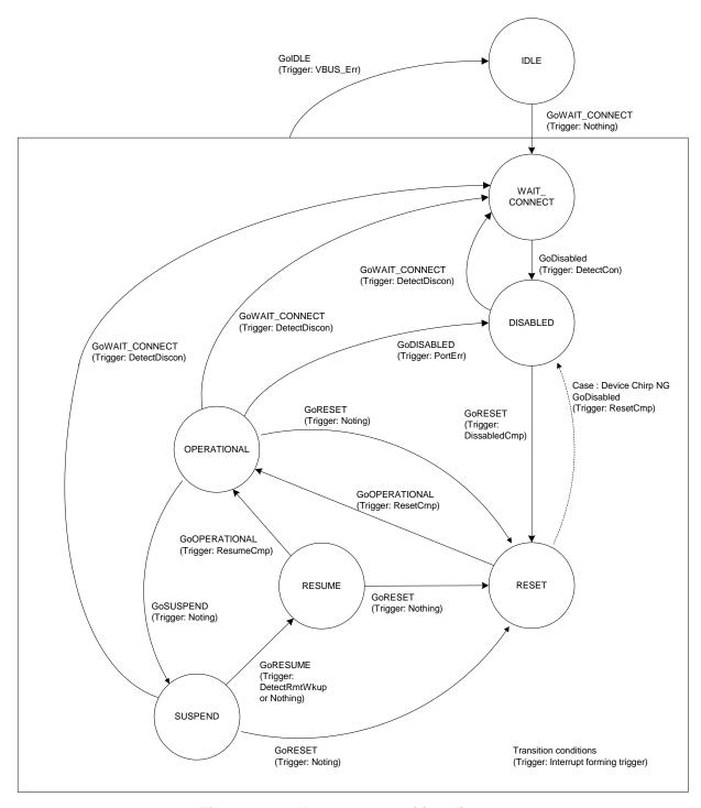
Figure 1-39 Host state transition diagram
