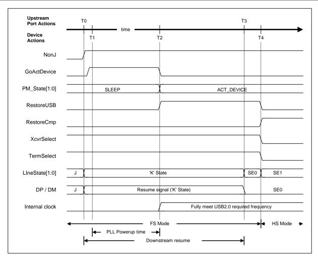
Figure 1-17 Detect resume timing (HS mode)
