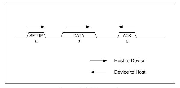
Figure 1-25 SETUP transaction
