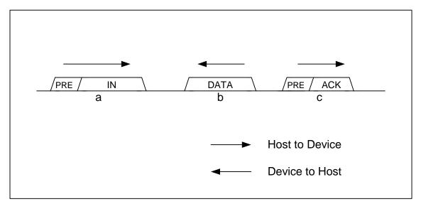
Figure 1-32 IN transaction with preamble attached
