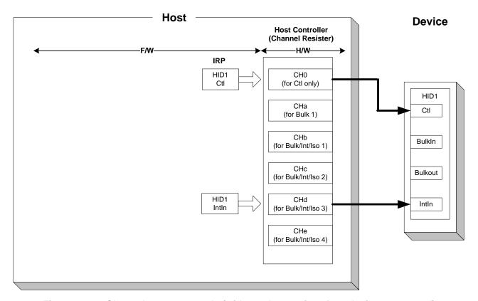
Figure 1-23 Channel usage example (with one human interface device connected)
