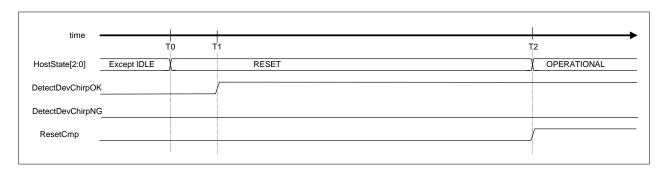
Figure 1-69 GoRESETtoOP timing (HS mode)
