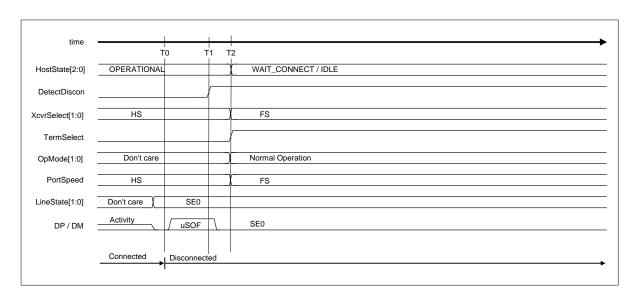
Figure 1-41 Disconnect detection timing (HS mode)
