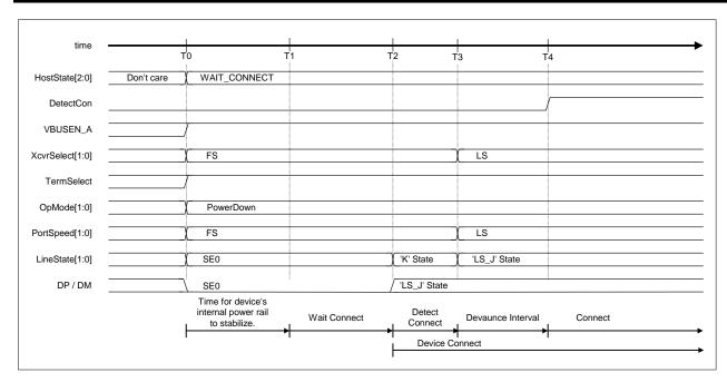
Figure 1-50 Device attach timing (LS mode)
