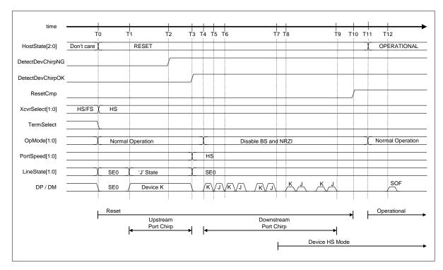
Figure 1-56 Detect device chirp NG timing (with chirp completion disable set to 1)
