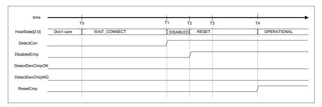
Figure 1-68 GoWAIT\_CONNECTtoOP timing (FS or LS mode)
