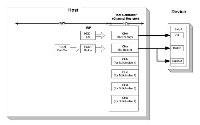
Figure 1-21 Channel usage example (with one storage device connected)
