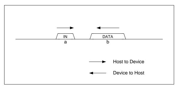
Figure 1-29 Isochronous IN transaction
