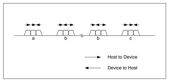
Figure 1-35 Control transfers with data stage in the IN direction
