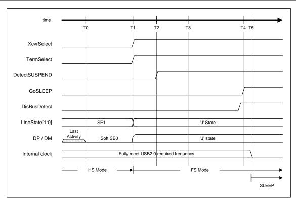
Figure 1-9 Suspend timing (HS mode)
