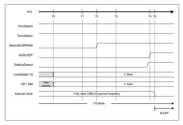
Figure 1-10 Suspend timing (FS mode)
