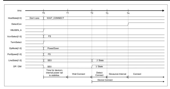
Figure 1-49 Device attach timing (FS mode)
