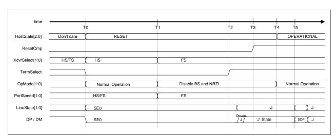
Figure 1-57 Reset timing (FS mode)
