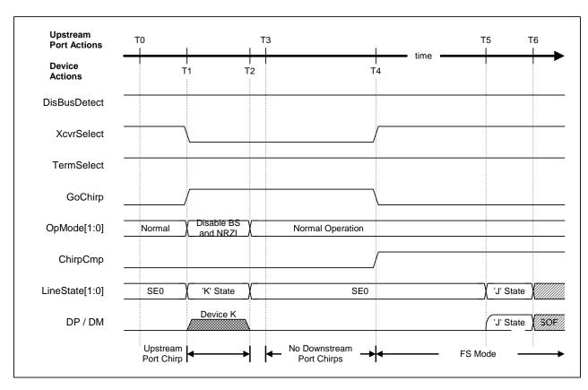
Figure 1-13 HS detection handshake timing (FS mode)
