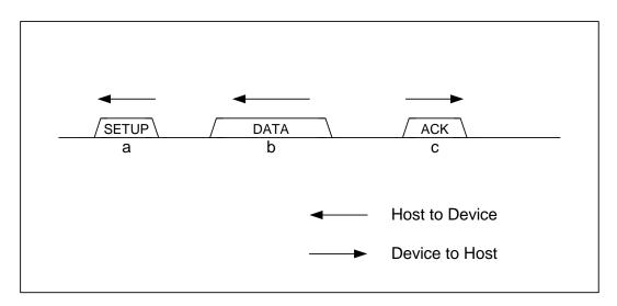
Figure 1-2 SETUP transaction
