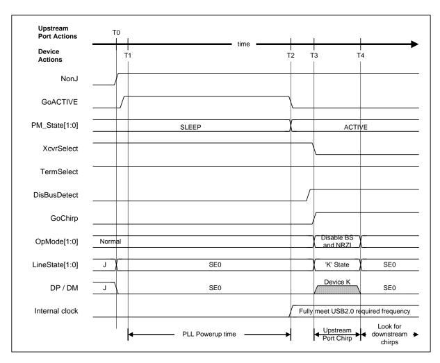
Figure 1-15 HS detection handshake timing from suspend
