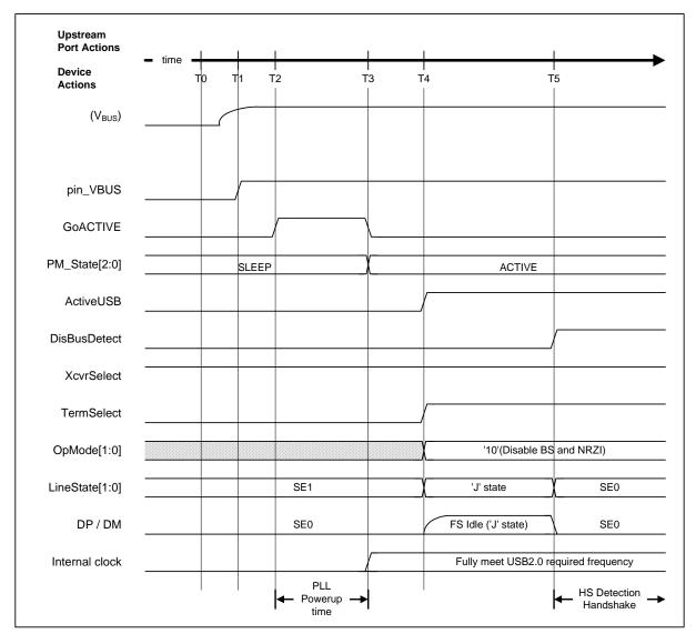
Figure 1-18 Device attach timing
