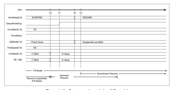
Figure 1-43 Remote wakeup timing (HS mode)
