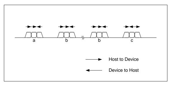
Figure 1-34 Control transfer with data stage in OUT direction
