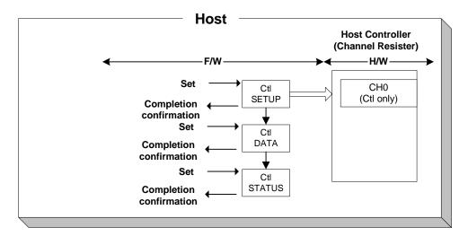
Figure 1-33 Control transfer control
