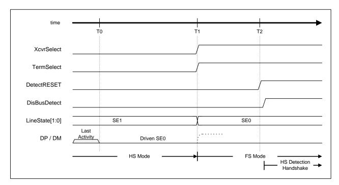
Figure 1-11 Reset timing (HS mode)
