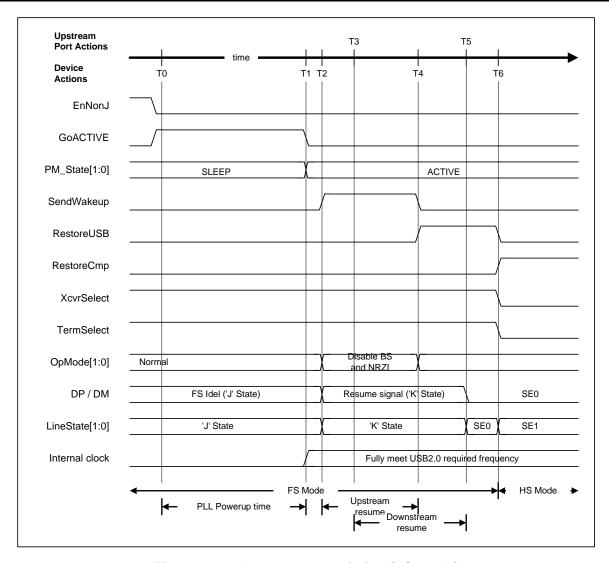
Figure 1-16 Assert resume timing (HS mode)
