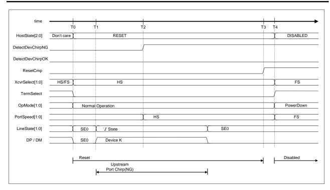
Figure 1-55 Detect device chirp NG timing (with chirp completion disable set to 0)
