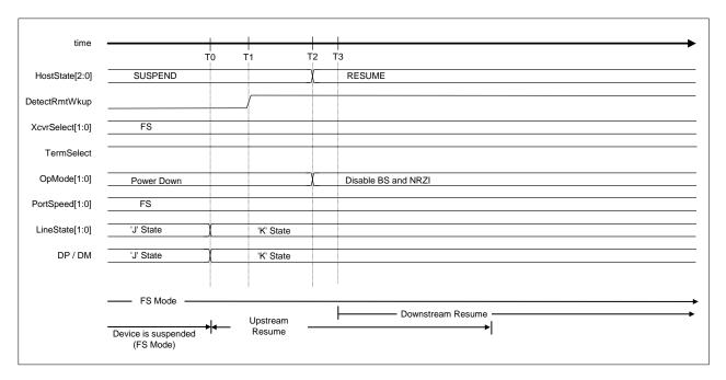
Figure 1-44 Remote wakeup timing (FS mode)
