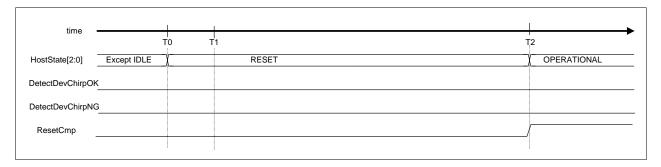
Figure 1-70 GoRESETtoOP timing (FS or LS mode)
