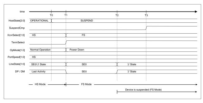
Figure 1-60 Suspend timing (HS mode)
