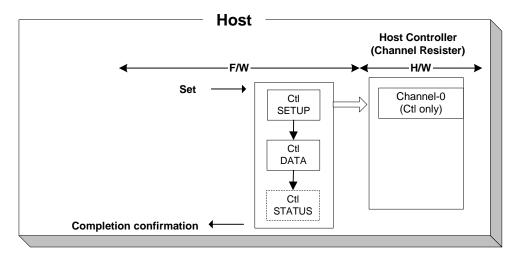
Figure 1-36 Control transfer support function control
