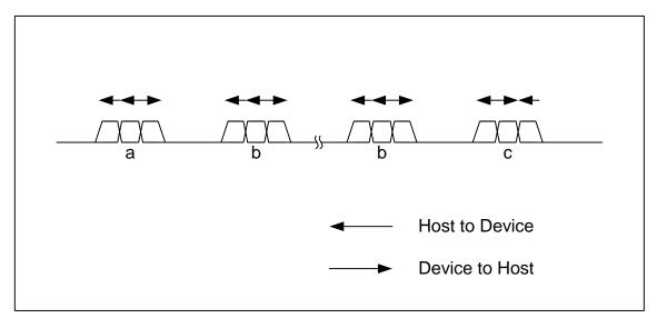
Figure 1-6 Control transfers when data stage is OUT
