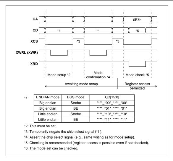
Figure 1-76 CPUIF mode setup
