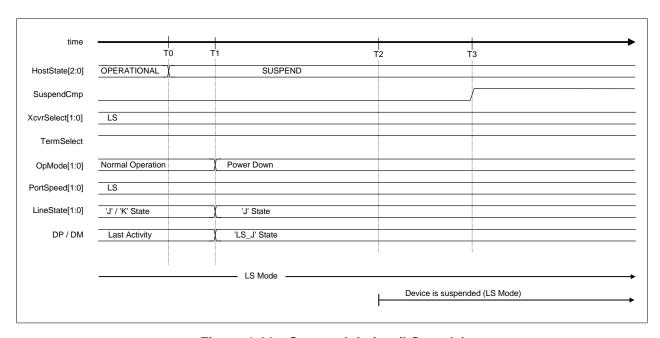
Figure 1-62 Suspend timing (LS mode)
