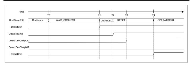
Figure 1-67 GoWAIT\_CONNECTtoOP timing (HS mode)
