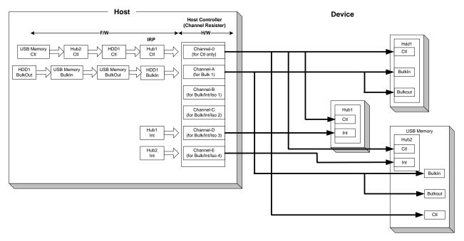
Figure 1-24 Channel usage example (with two storage devices connected via a hub)
