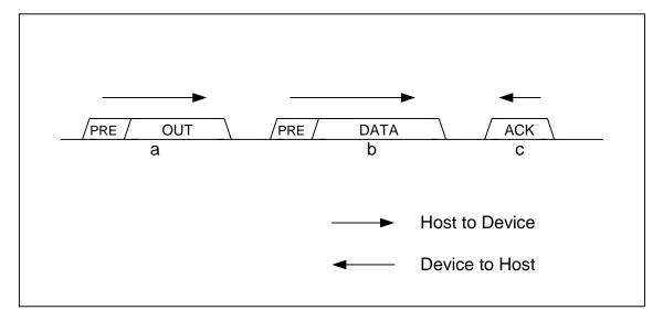
Figure 1-31 OUT transaction with preamble attached
