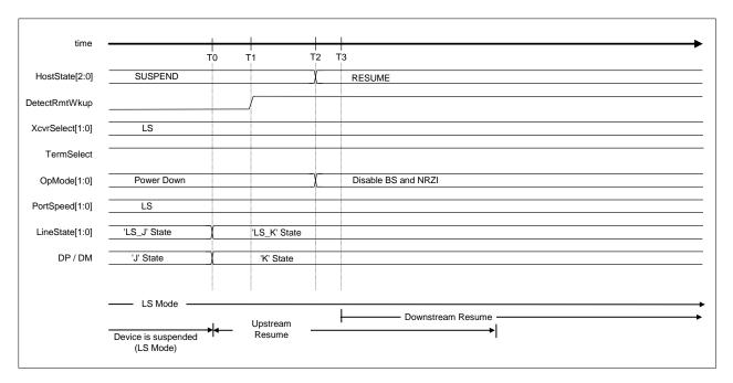
Figure 1-45 Remote wakeup timing (LS mode)
