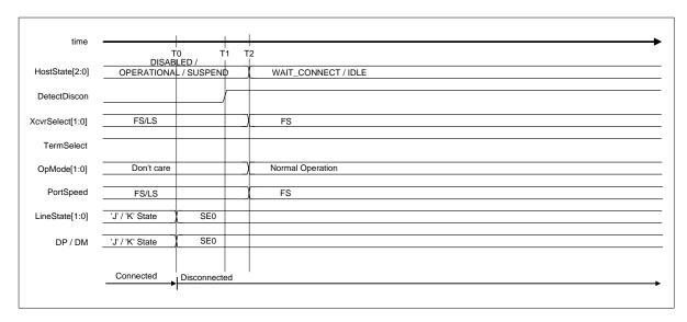
Figure 1-42 Disconnect detection timing (FS or LS mode)
