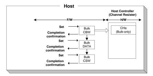
Figure 1-38 Control when not using bulk-only support function (reference)
