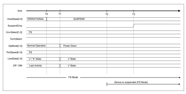
Figure 1-61 Suspend timing (FS mode)
