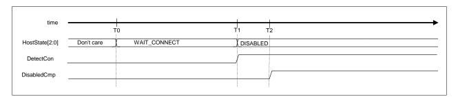
Figure 1-66 GoWAIT\_CONNECTtoDIS timing (HS mode)
