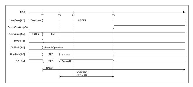
Figure 1-46 Device chirp timing
