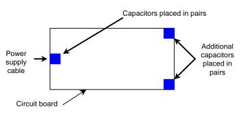
(4) Install bypass capacitors close to all power pins.
