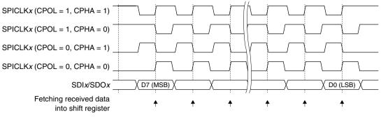
Figure 16.4.1 Clock and Data Transfer Timing
