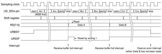
Figure 19.5.1.2 Data Receiving Timing Chart (UART mode)
