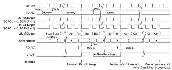
Figure 19.5.2.2 Data Receiving Timing Chart (SPI master mode)
