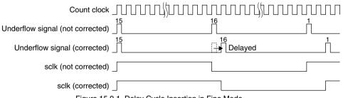
Figure 15.9.1 Delay Cycle Insertion in Fine Mode
