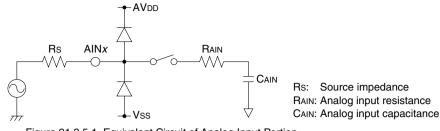
Figure 21.3.5.1 Equivalent Circuit of Analog Input Portion
