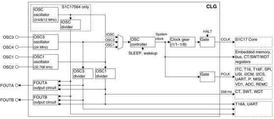
Figure 7.1.1 CLG Module Configuration
