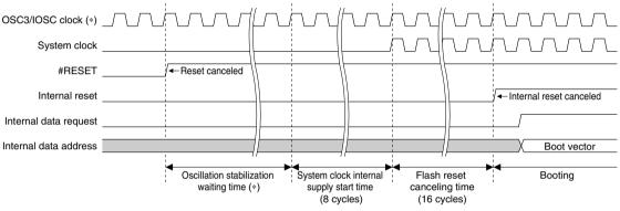
Figure 5.2.1 Operation Sequence Following Cancellation of Initial Reset
