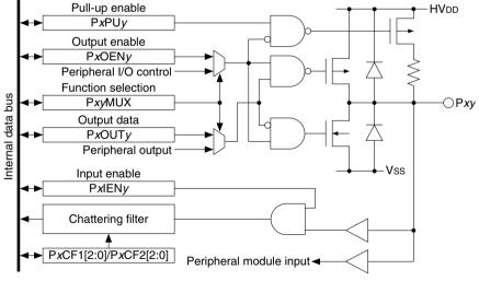
Figure 8.1.1 I/O Port Configuration
