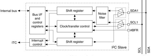
Figure 18.1.1 I2CS Module Configuration
