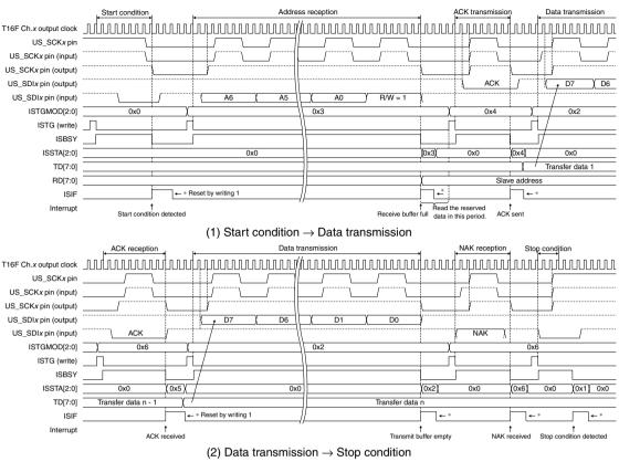
Figure 19.5.3.13 I<sup>2</sup>C Slave Data Transmission Timing Chart
