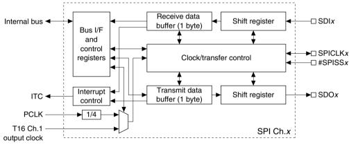
Figure 16.1.1 SPI Module Configuration (1 channel)
