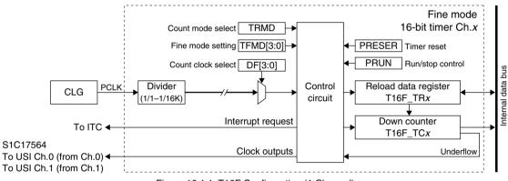
Figure 10.1.1 T16F Configuration (1 Channel)
