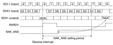
Figure 18.5.3 NAK\_ANS Setting and NAK Response Timing
