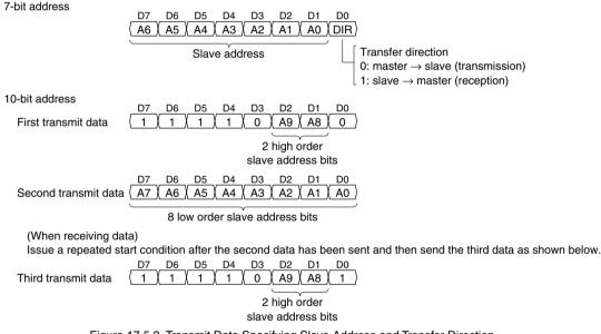
Figure 17.5.2 Transmit Data Specifying Slave Address and Transfer Direction
