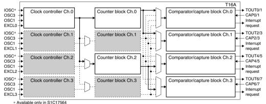
(1) Configuration Example 1 (four comparator/capture blocks × two channels)
