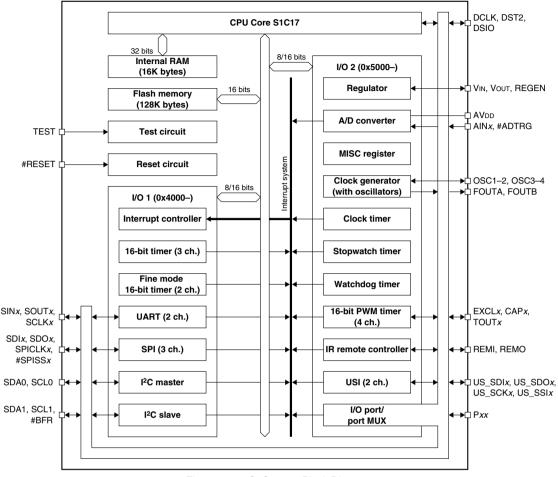
Figure 1.2.2 S1C17564 Block Diagram
