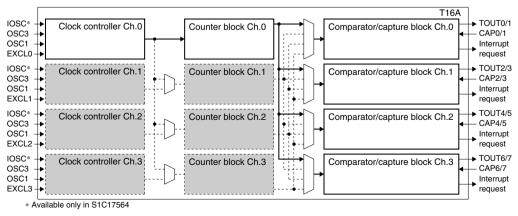
(2) Configuration Example 2 (eight comparator/capture blocks  $\times$  one channel) Figure 11.4.3.2 Timer Configuration Example in Multi-Comparator/Capture Mode
