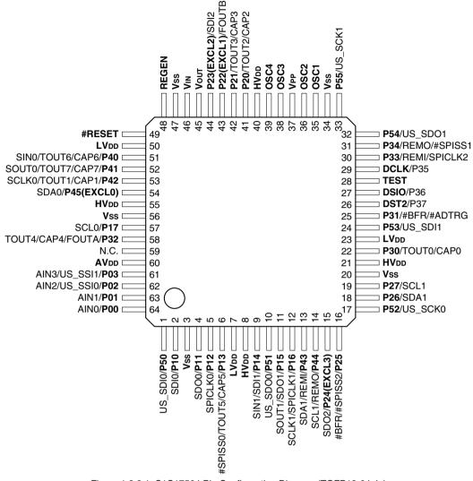
Figure 1.3.2.1 S1C17564 Pin Configuration Diagram (TQFP13-64pin)
