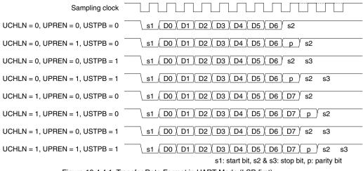
Figure 19.4.4.1 Transfer Data Format in UART Mode (LSB first)
