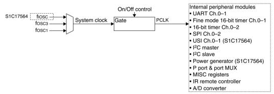
Figure 7.6.1 Peripheral Module Clock Control Circuit
