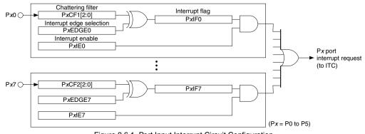
Figure 8.6.1 Port Input Interrupt Circuit Configuration
