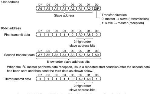
Figure 19.5.3.5 Transmit Data Specifying Slave Address and Transfer Direction
