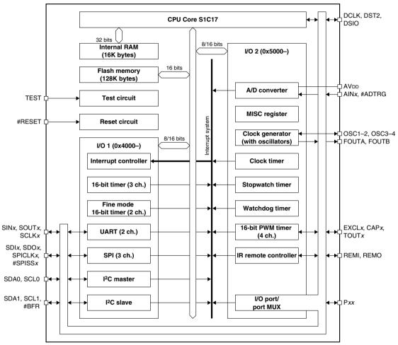
Figure 1.2.1 S1C17554 Block Diagram
