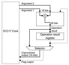
Figure 23.3.1 Data Path in Multiplication Mode
