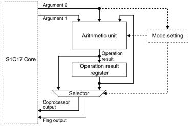
Figure 23.1.1 Multiplier/Divider Block Diagram
