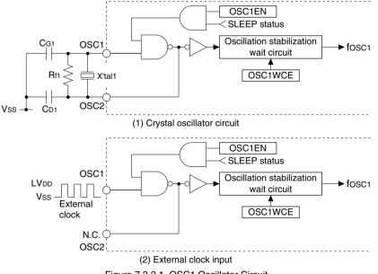
Figure 7.3.2.1 OSC1 Oscillator Circuit
