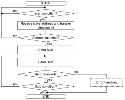
Figure 19.5.3.12 I<sup>2</sup>C Slave Data Transmission Flow Chart
