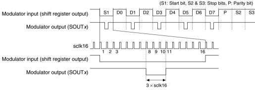
Figure 15.8.1 Transmission Signal Waveform
