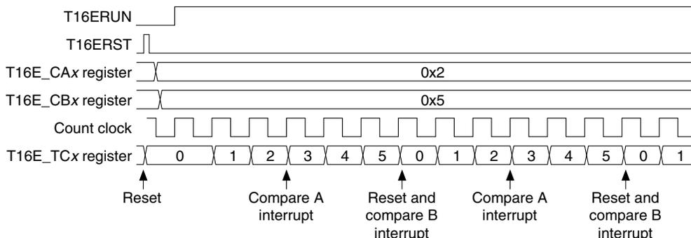
Figure 12.6.1 Basic Counter Operation Timing
