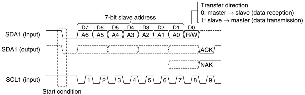
Figure 21.5.1 Receiving Slave Address and Data Direction Bit
