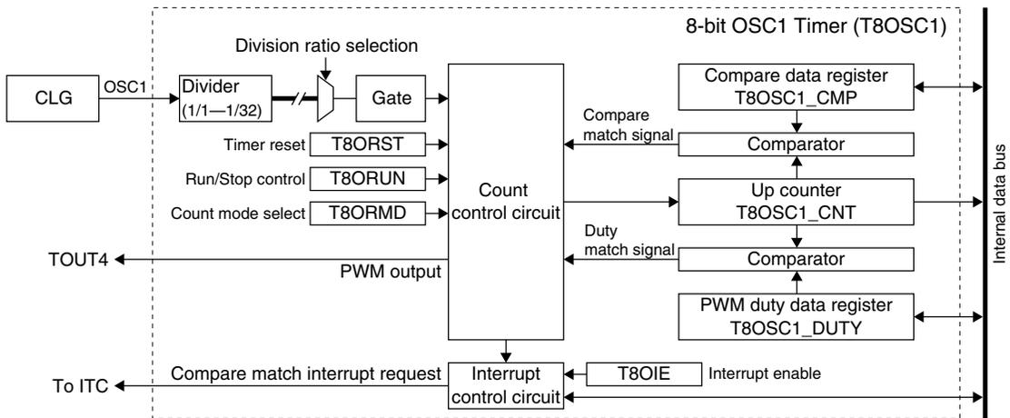
Figure 14.1.1 T8OSC1 Module Configuration
