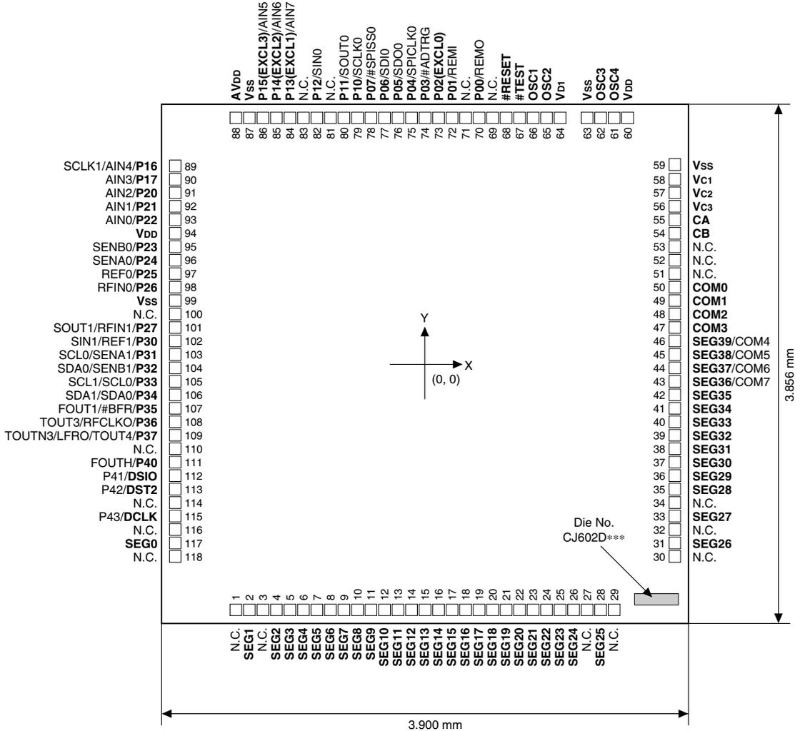
Figure 1.3.4.3 S1C17602/621 Pad Configuration Diagram
