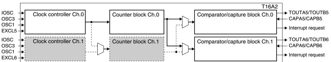
Figure 13.4.3.2 Timer Configuration in Multi-Comparator/Capture Mode
