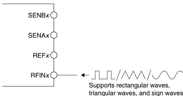
Figure 25.4.2.1 External Clock Input
