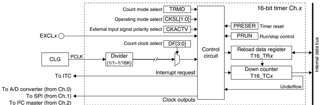
Figure 11.1.1 T16 Configuration (1 Channel)
