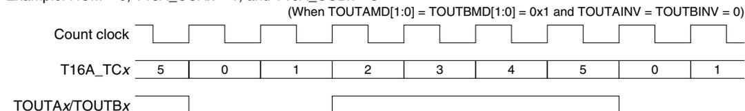
Figure 13.6.3 PWM Waveform Output Timings in Normal Clock Mode
