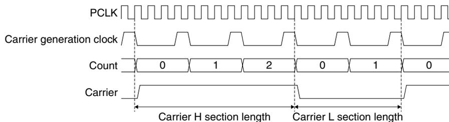
Figure 22.3.1 Carrier Signal Generation
