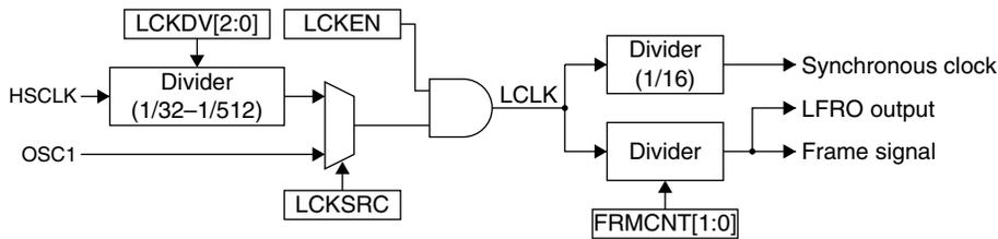
Figure 23.3.1 LCD Clock System
