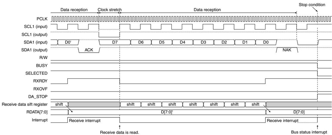
Figure 21.5.8 I2CS Timing Chart 4 (data reception → stop condition)
