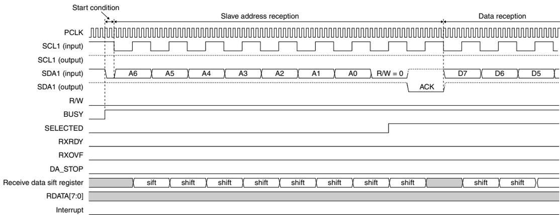
Figure 21.5.7 I2CS Timing Chart 3 (start condition → data reception)
