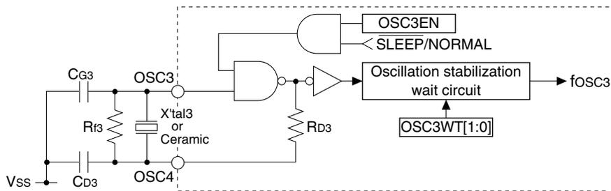
Figure 7.3.2.1 OSC3 Oscillator Circuit
