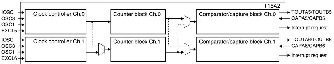
Figure 13.4.3.1 Timer Configuration in Normal Channel Mode
