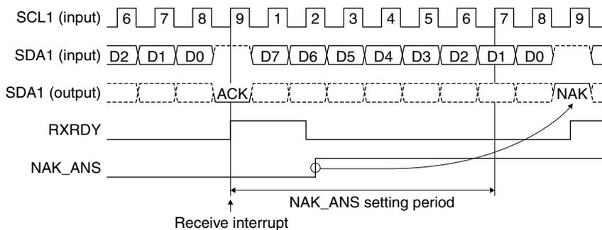
Figure 21.5.3 NAK\_ANS Setting and NAK Response Timing
