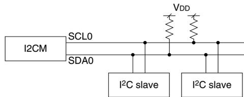
Figure 20.2.1 I<sup>2</sup>C Connection Example
