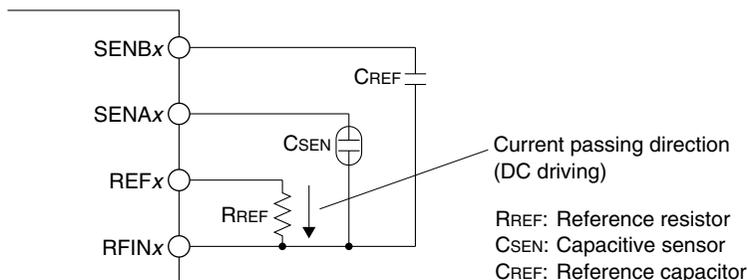
Figure 25.4.1.3 Connection Example in DC Oscillation Mode for Measuring Capacitive Sensors
