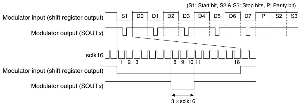
Figure 18.8.1 Transmission Signal Waveform
