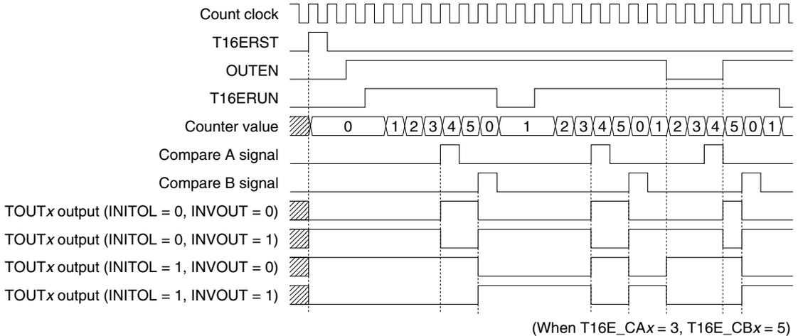
Figure 12.7.2 T16E Output Waveform
