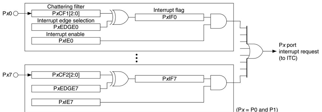
Figure 9.7.1 Port Input Interrupt Circuit Configuration
