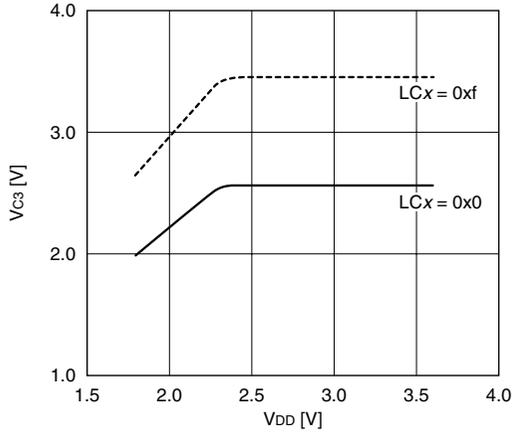
**LCD drive voltage-supply voltage characteristic (when Vc1 reference voltage is selected)**
