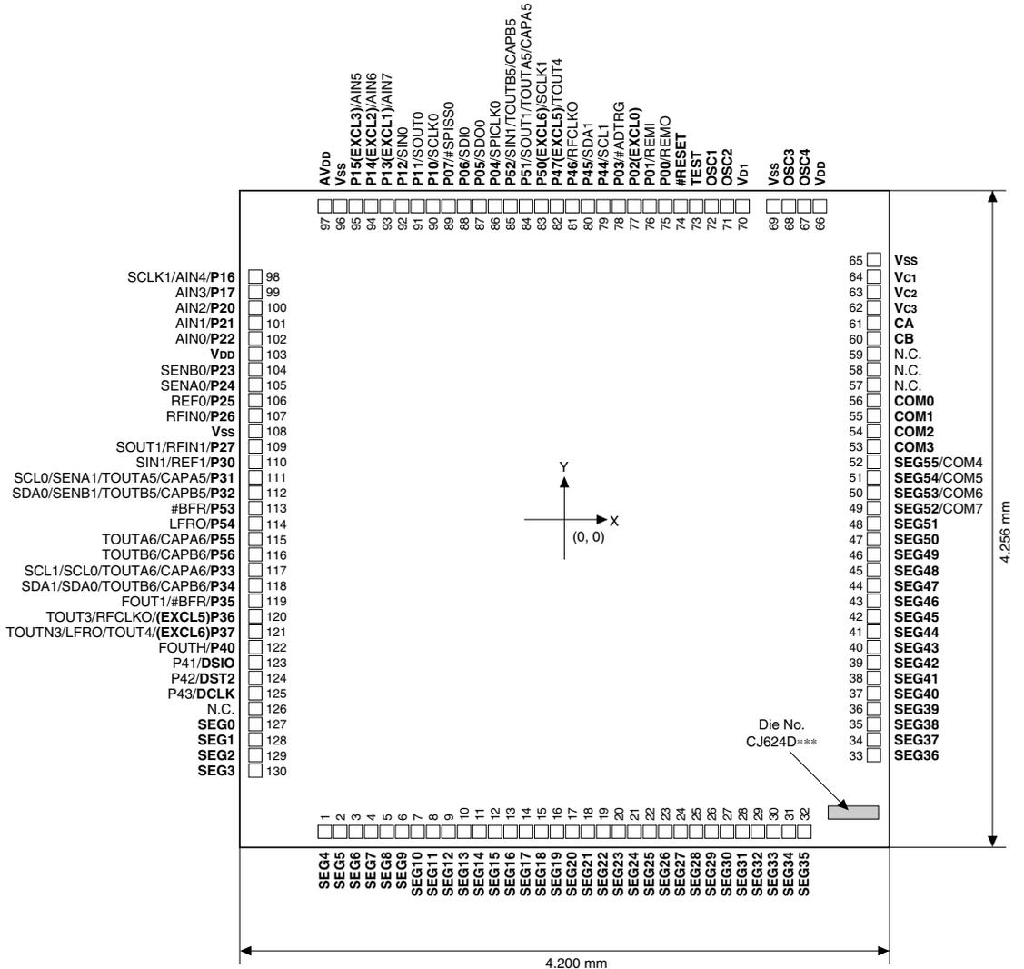
Figure 1.3.1.2 S1C17624 Pad Configuration Diagram
