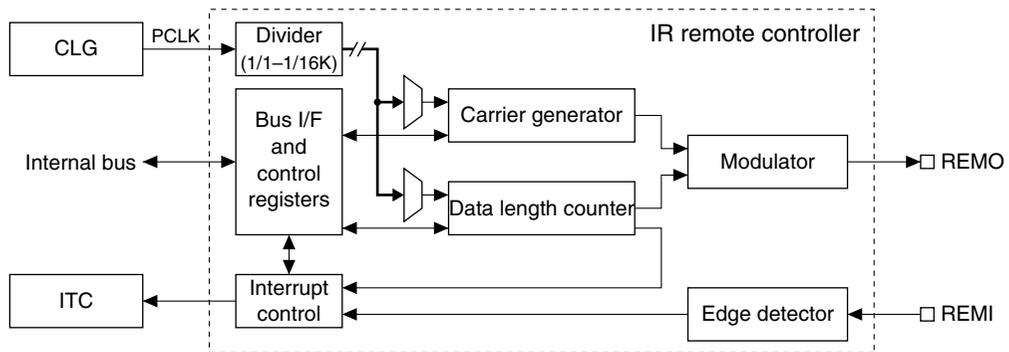
Figure 22.1.1 REMC Module Configuration
