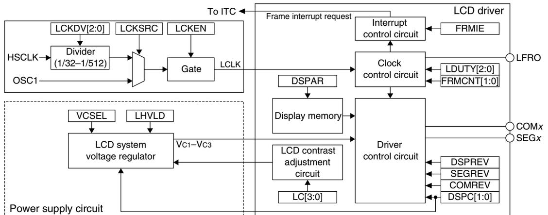
Figure 23.1.1 LCD Driver and Driver Power Supply Configuration
