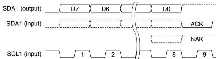
Figure 21.5.2 ACK and NAK
