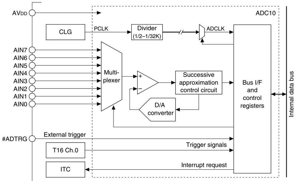
Figure 24.1.1 A/D Converter Configuration
