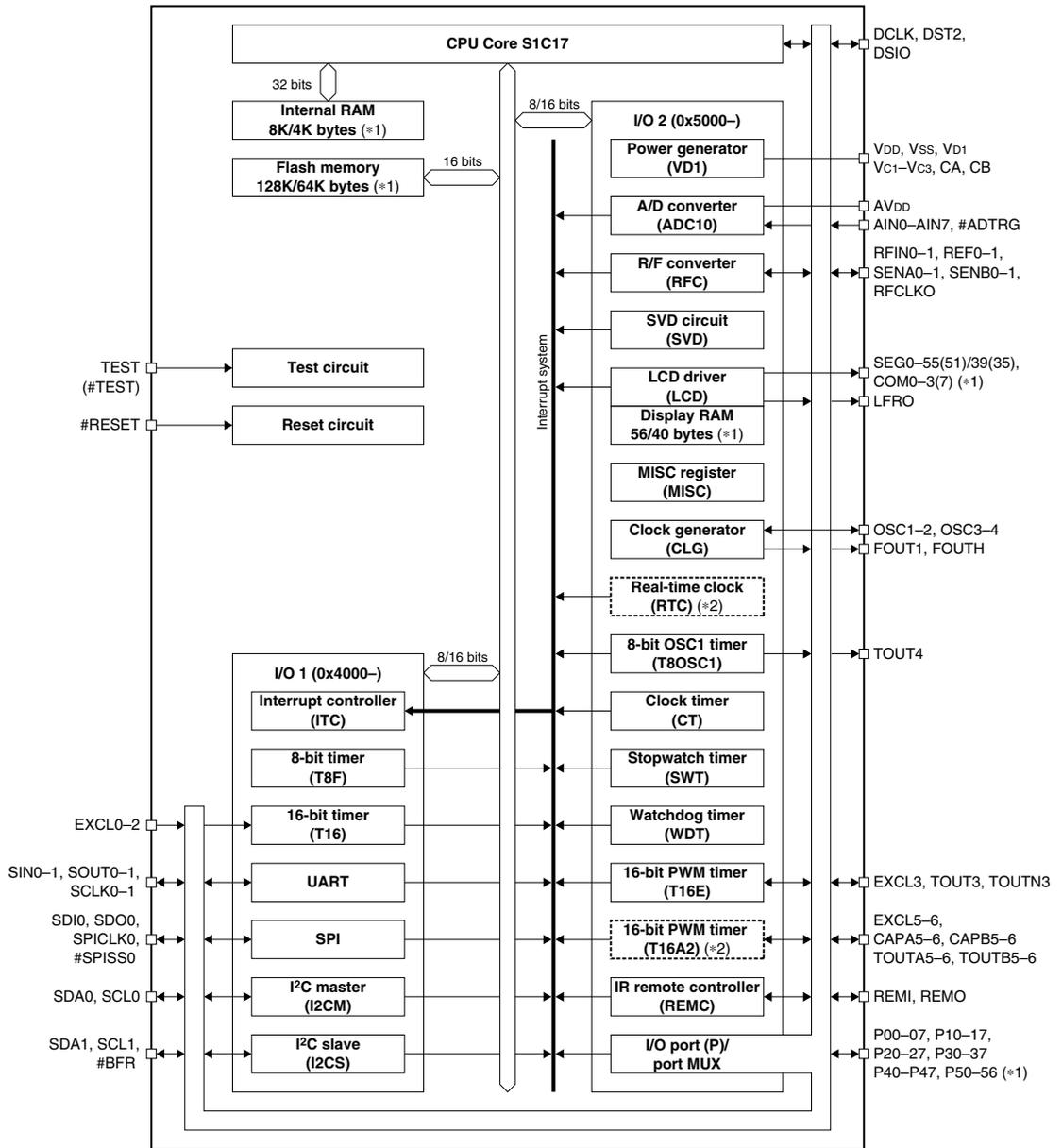
Figure 1.2.1 Block Diagram
