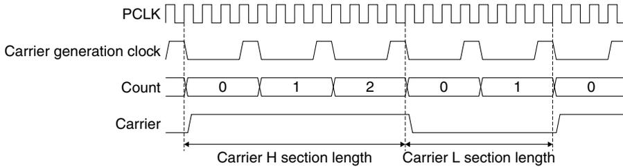
Figure 22.7.1 Carrier Signal Generation
