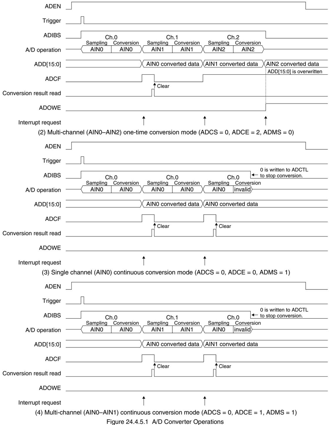
Figure 24.4.5.1 A/D Converter Operations
