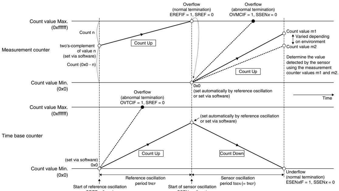
Figure 25.6.2.1 Counter Operations During Reference/Sensor Oscillation
