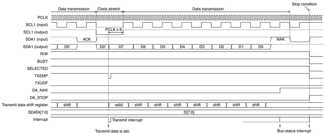
Figure 21.5.6 I2CS Timing Chart 2 (data transmission → stop condition)
