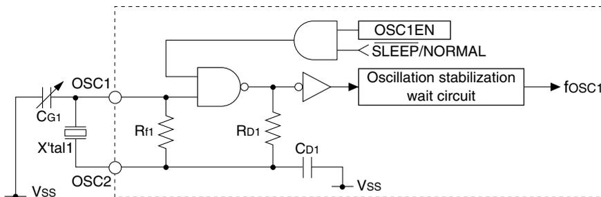
Figure 7.3.3.1 OSC1 Oscillator Circuit (S1C17622/602/621)
