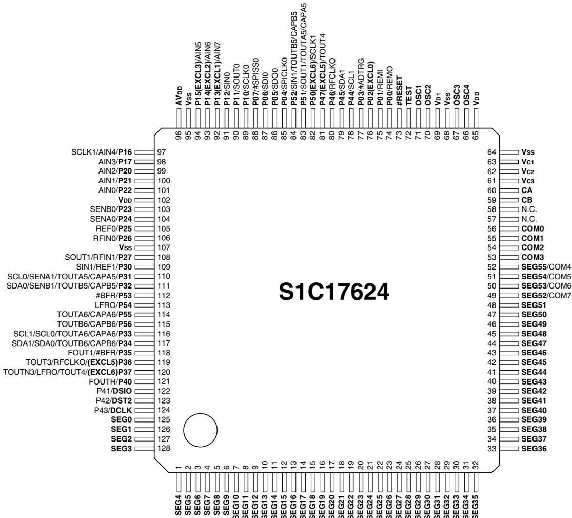
Figure 1.3.1.1 S1C17624 Pin Configuration Diagram (TQFP15-128pin)
