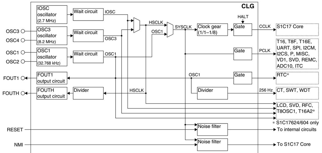
Figure 7.1.1 CLG Module Configuration
