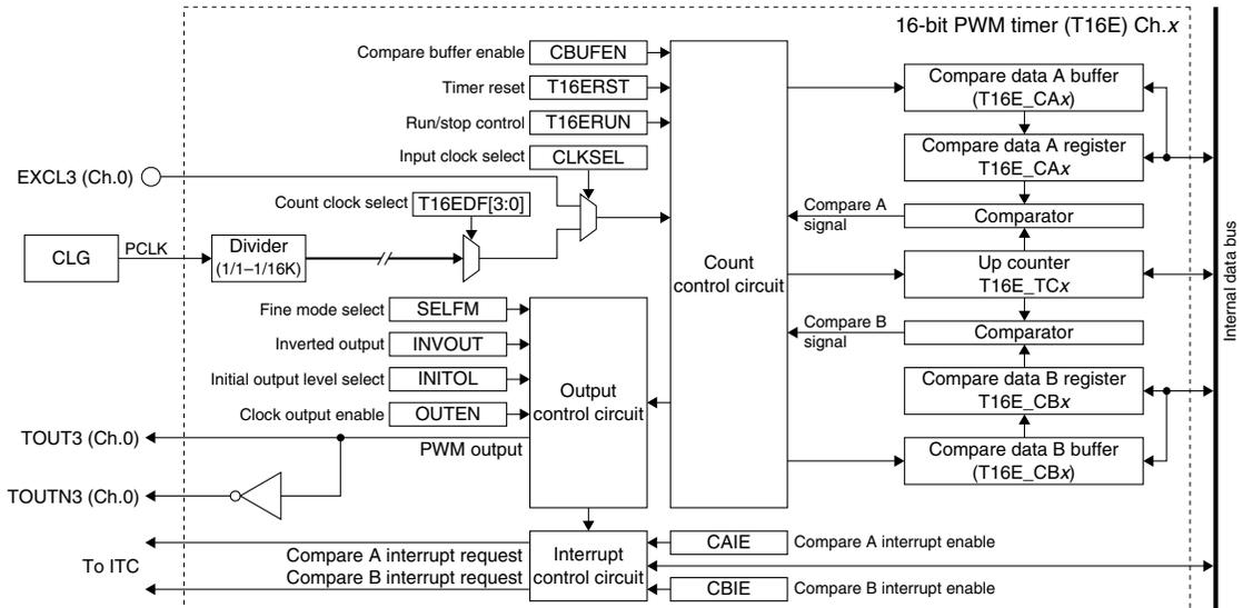
Figure 12.1.1 T16E Module Configuration
