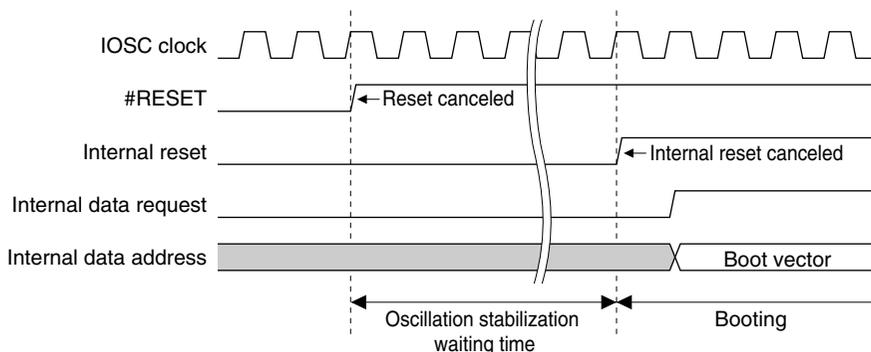
Figure 5.2.1 Operation Sequence Following Cancellation of Initial Reset
