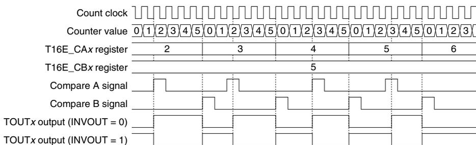
Figure 12.7.3 Fine Mode Clock Output
