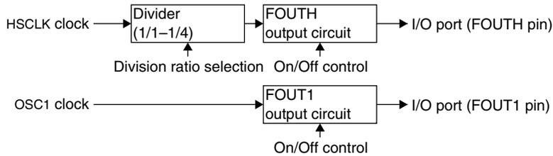
Figure 7.7.1 Clock Output Circuit
