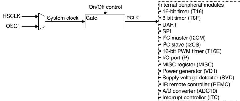
Figure 7.6.1 Peripheral Module Clock Control Circuit
