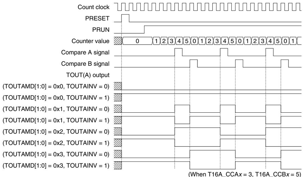
Figure 13.6.2 TOUT Output Waveform
