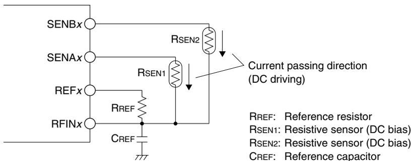
Figure 25.4.1.1 Connection Example in DC Oscillation Mode for Measuring Resistive Sensors
