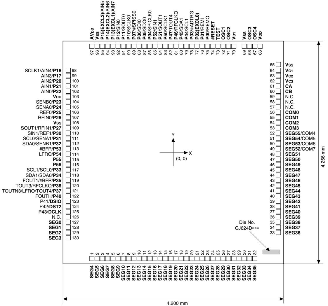
Figure 1.3.3.2 S1C17622 Pad Configuration Diagram
