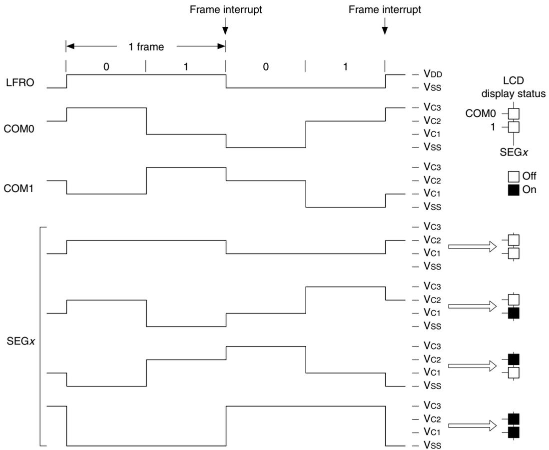
Figure 23.4.2.4 1/2 Duty Drive Waveform
