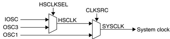
Figure 7.4.1 System Clock Selector
