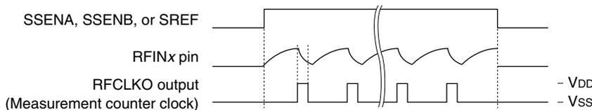
Figure 25.4.3.1 CR Oscillation Clock (RFCLK) Waveform
