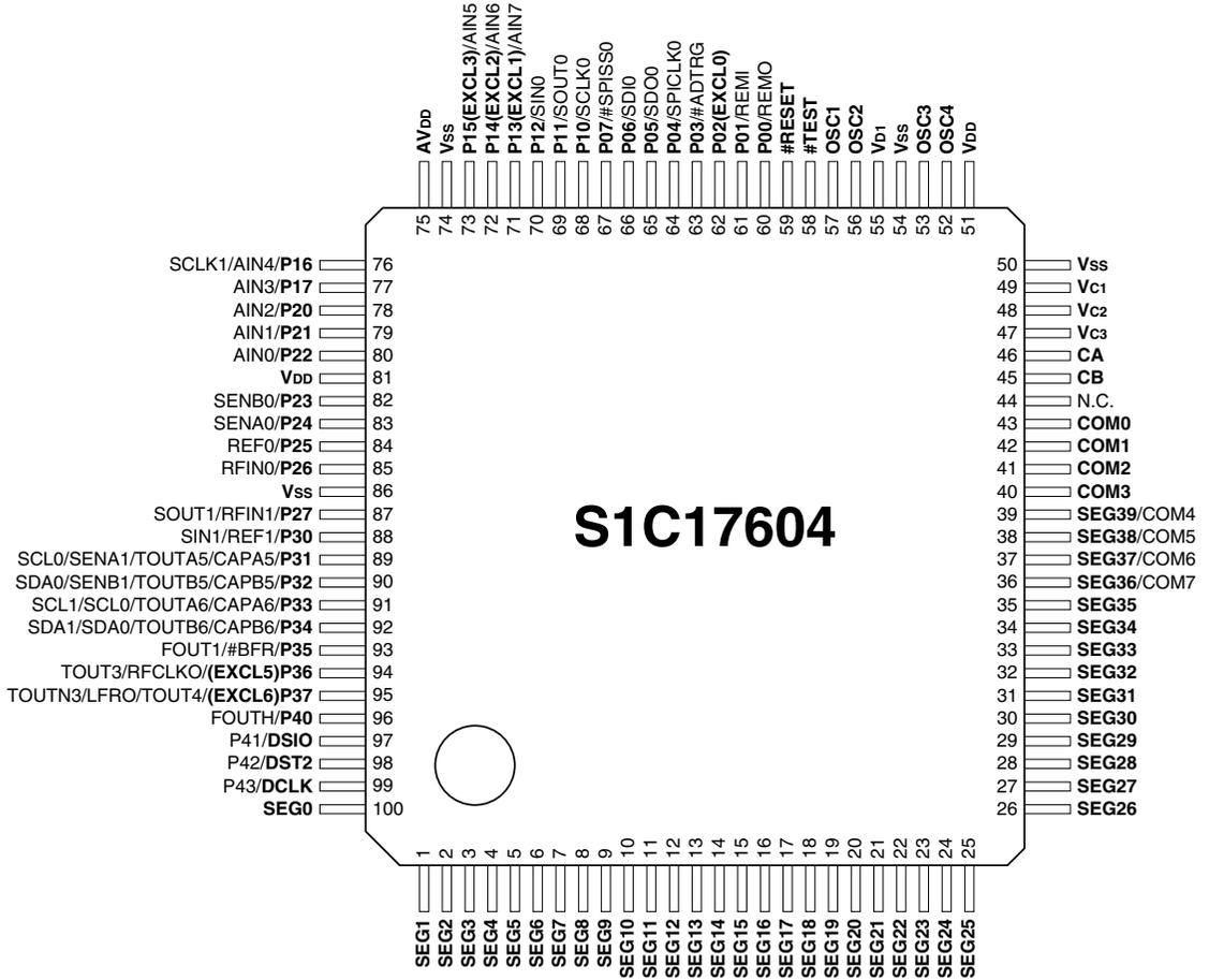
Figure 1.3.2.1 S1C17604 Pin Configuration Diagram (TQFP14-100pin)
