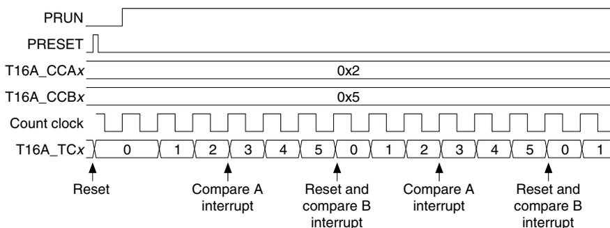
Figure 13.5.4.1 Operation Timing in Comparator Mode
