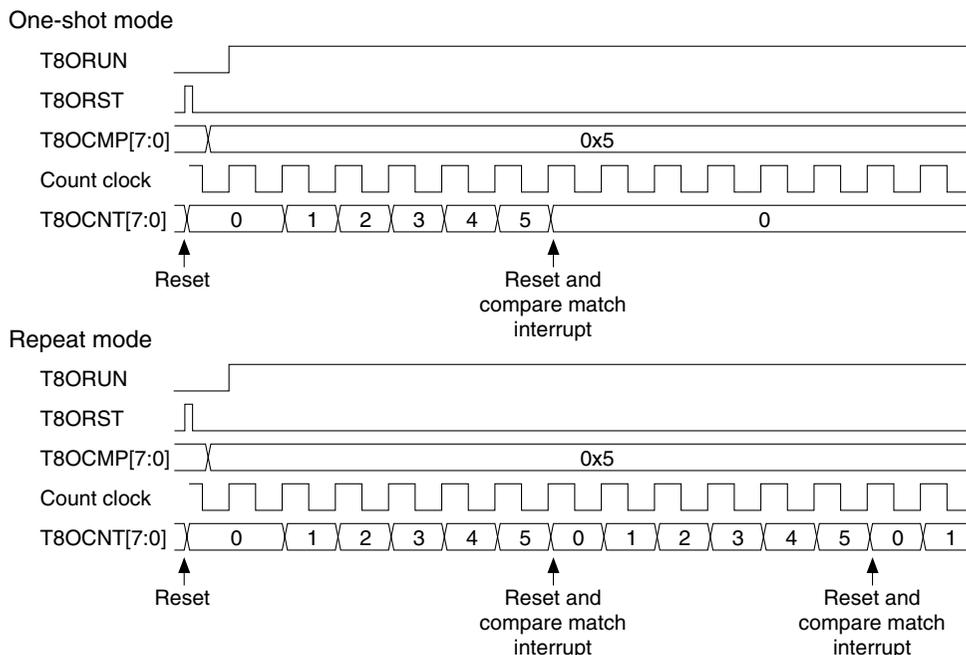
Figure 14.7.1 Basic Counter Operation Timing
