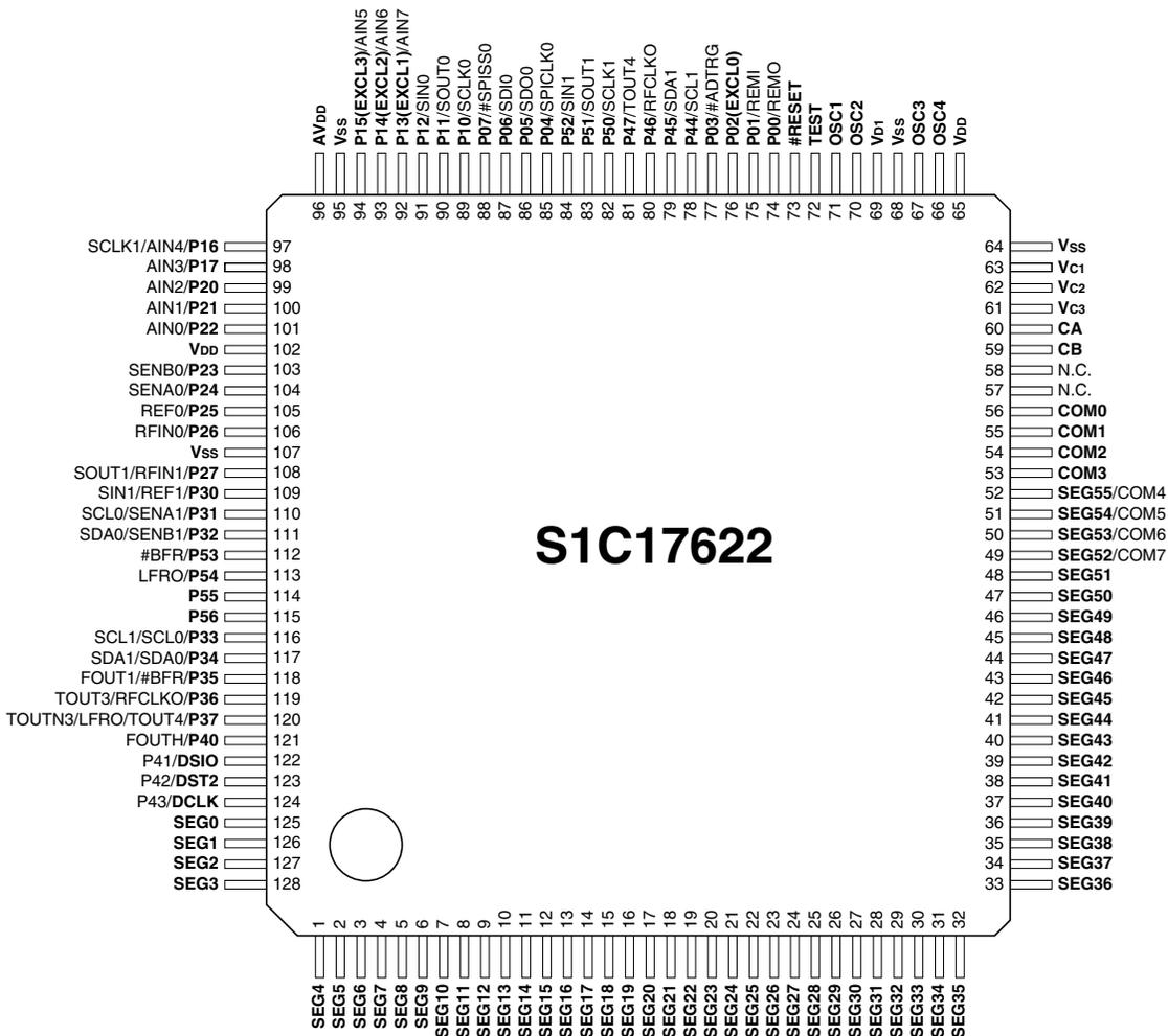
Figure 1.3.3.1 S1C17622 Pin Configuration Diagram (TQFP15-128pin)
