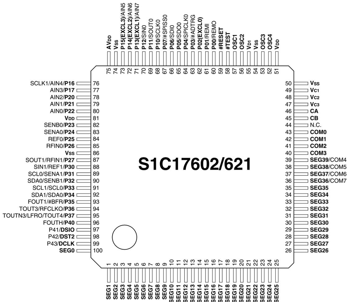
Figure 1.3.4.1 S1C17602/621 Pin Configuration Diagram (TQFP14-100pin)
