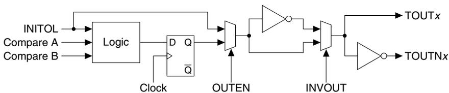
Figure 12.7.1 T16E Clock Output Circuit
