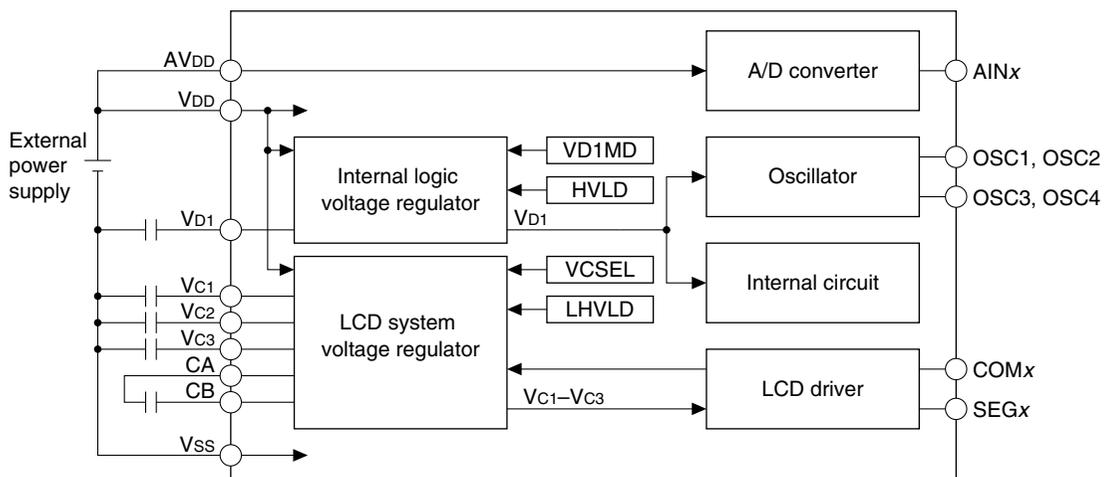
Figure 4.3.1 Configuration of Power Supply Circuit
