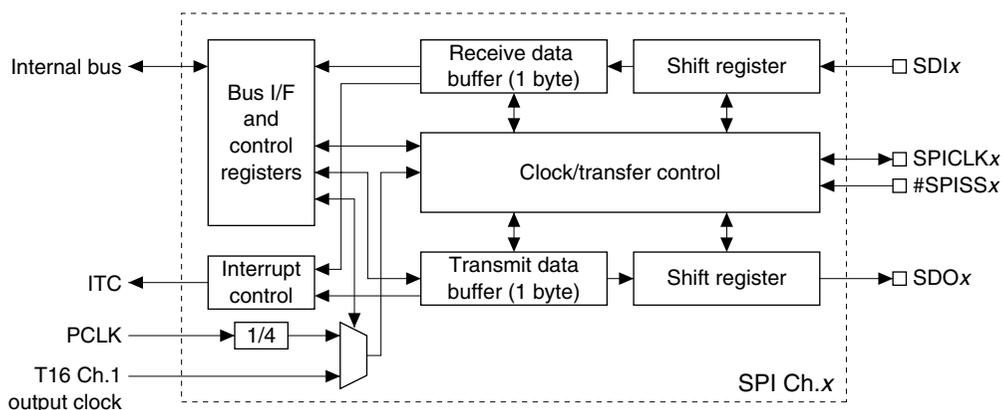
Figure 19.1.1 SPI Module Configuration
