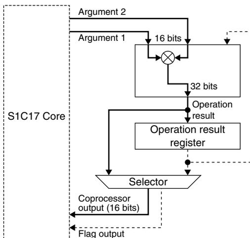
Figure 28.3.1 Data Path in Multiplication Mode
