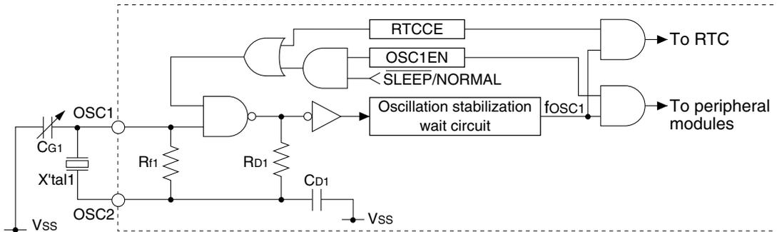
Figure 7.3.3.2 OSC1 Oscillator Circuit (S1C17624/604)
