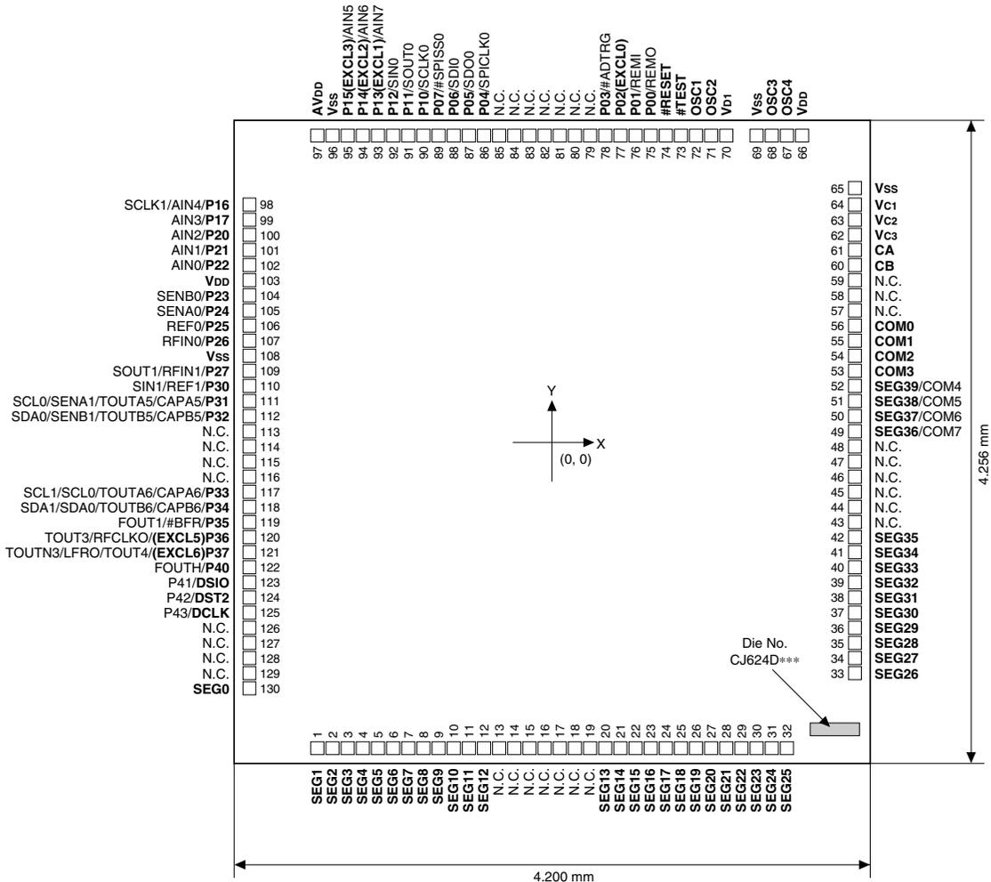
Figure 1.3.2.2 S1C17604 Pad Configuration Diagram
