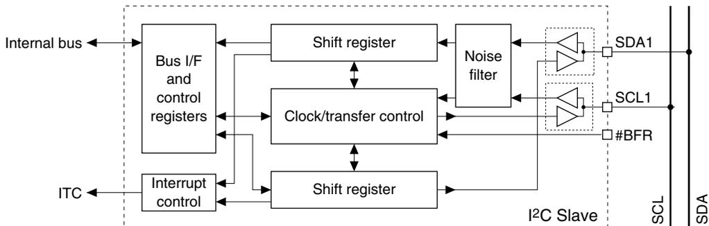
Figure 21.1.1 I2CS Module Configuration
