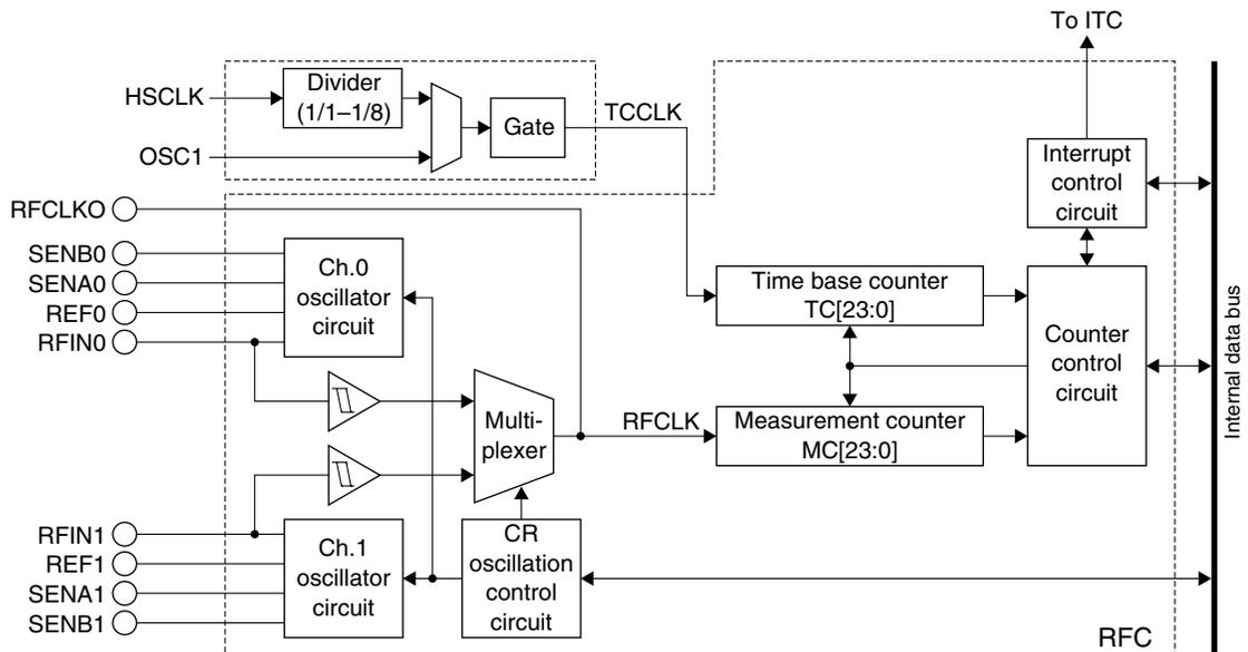
Figure 25.1.1 R/F Converter Configuration
