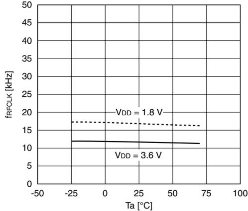
**RFC reference/sensor oscillation frequency-temperature characteristic**
