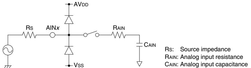
Figure 24.3.5.1 Equivalent Circuit of Analog Input Portion
