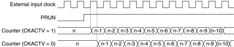
Figure 11.3.2.1 Counting in External Clock Mode
