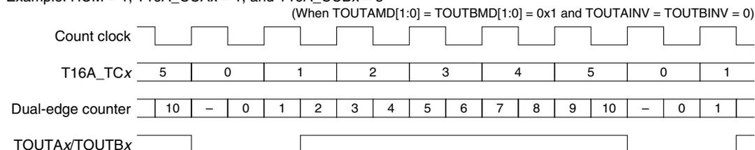
Figure 13.6.4 PWM Waveform Output Timings in Half Clock Mode
