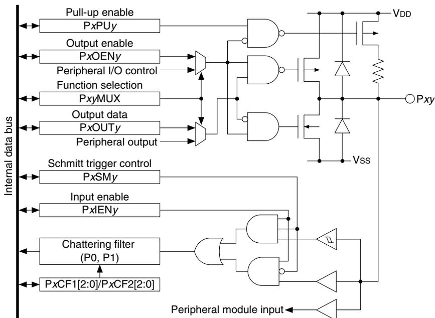
Figure 9.1.1 I/O Port Configuration
