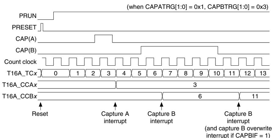
Figure 13.5.4.2 Operation Timing in Capture Mode
