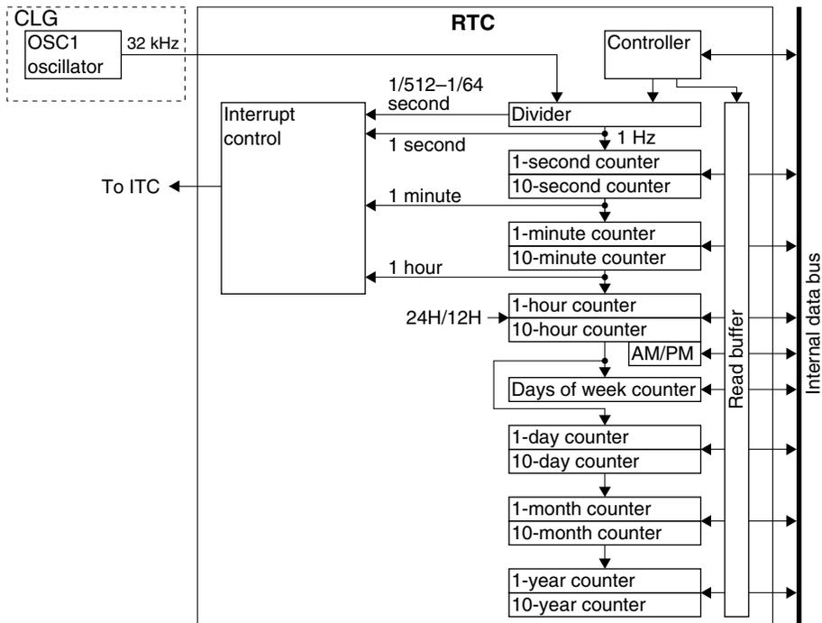
Figure 8.1.1 RTC Block Diagram
