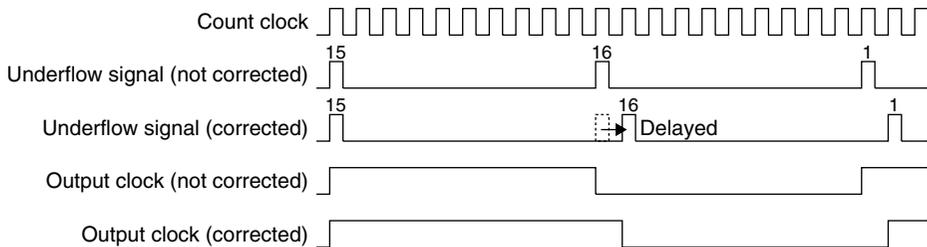
Figure 10.8.1 Delay Cycle Insertion in Fine Mode
