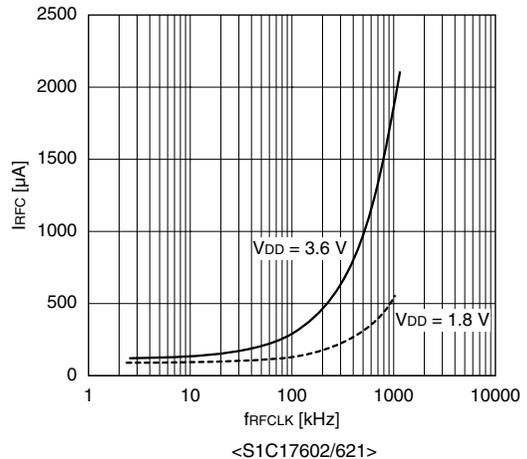
**RFC reference/sensor oscillation current consumption-frequency characteristic (Capacitive sensor DC oscillation mode)**
