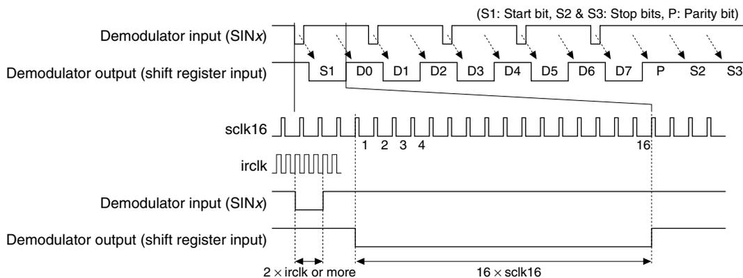
Figure 18.8.2 Receive Signal Waveform
