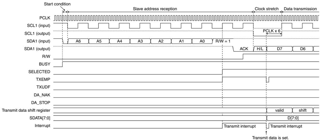
Figure 21.5.5 I2CS Timing Chart 1 (start condition → data transmission)
