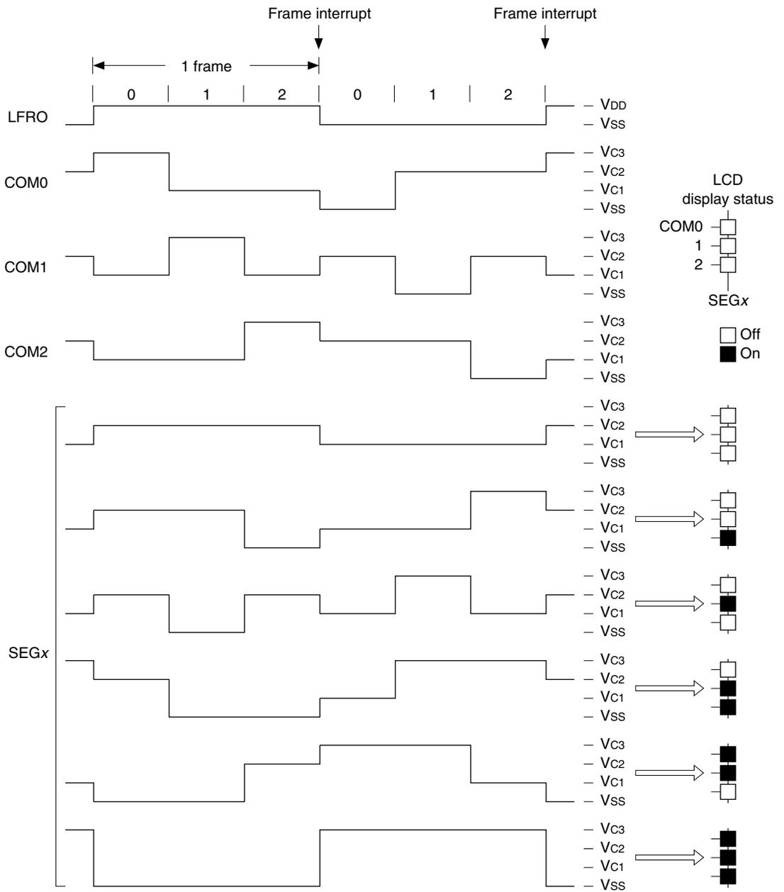
Figure 23.4.2.3 1/3 Duty Drive Waveform
