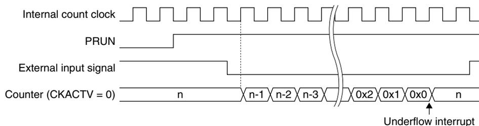
Figure 11.3.3.1 Count Operation in Pulse Width Measurement Mode
