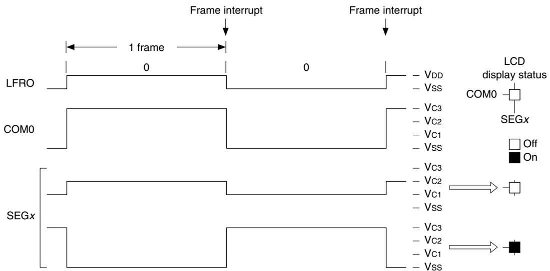
Figure 23.4.2.5 Static Drive Waveform
