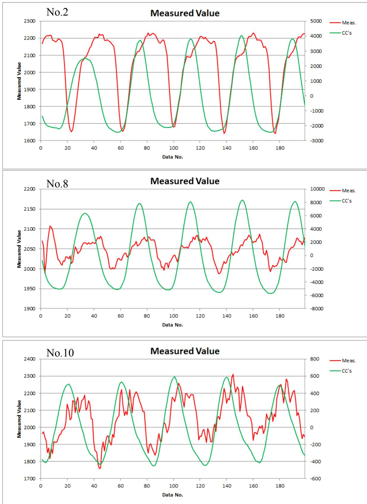
Figure A-2 Results with Square Wave Correlation Filtering Only
