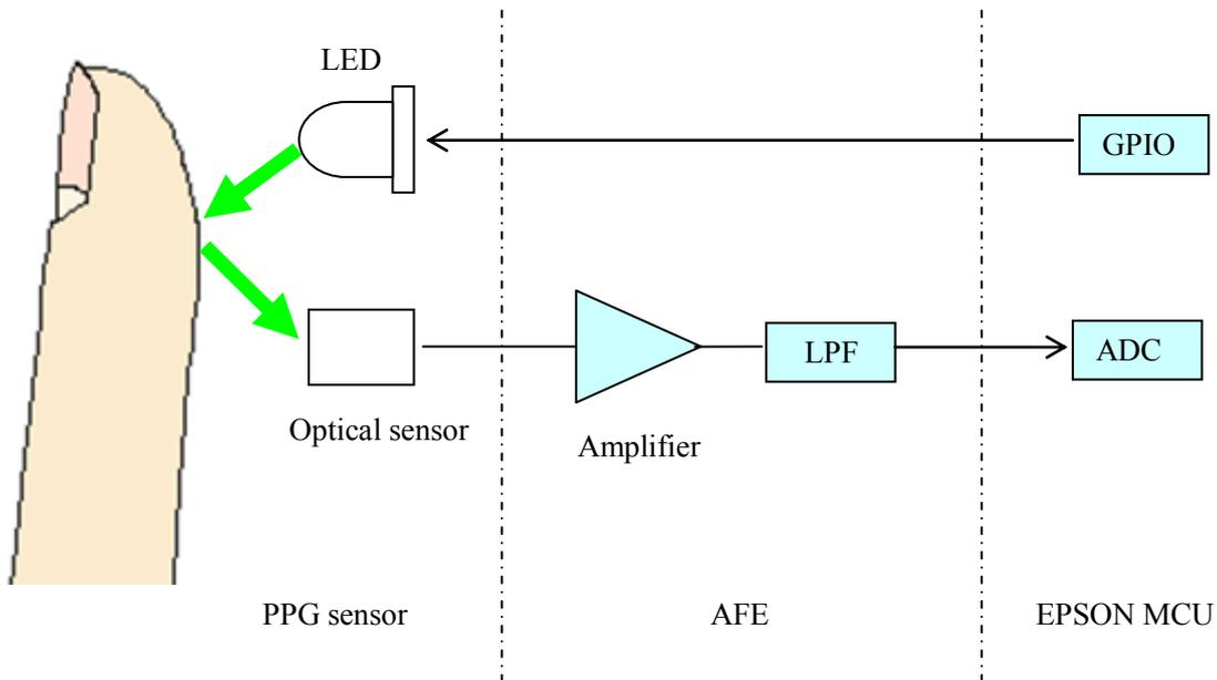
Figure 3-2 Circuit Block Diagram Used For Reflection Type Photoelectric Pulse Wave Measurement
