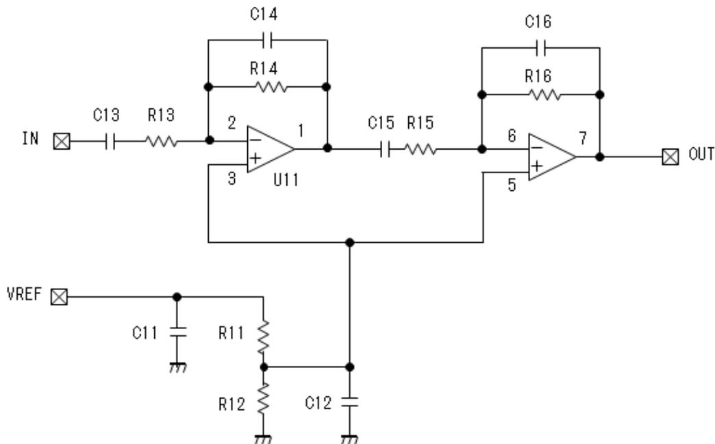
Figure 3-4 Example of Continuous-Drive Pulse Wave Detector AFE Circuit<sup>4)</sup>
