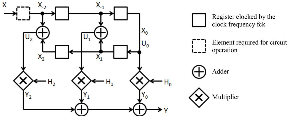
Figure 3-8 FIR Filter Configuration
