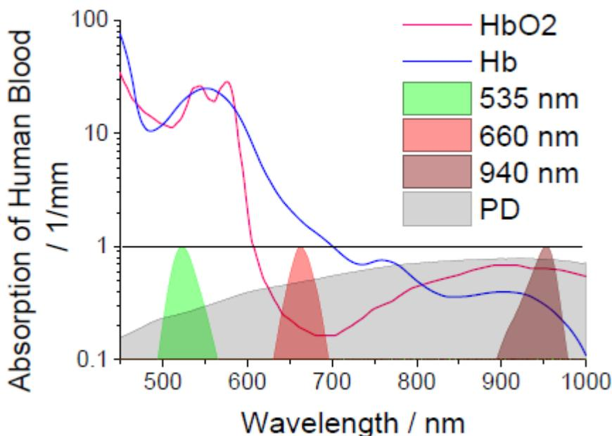
Figure 3-1 Absorption of Human Blood (Oxyhemoglobin and Hemoglobin) vs. Wavelength of Light <sup>2)</sup>
