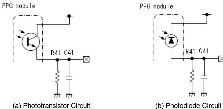
Figure 3-7 Examples of Optical Sensor Circuit
