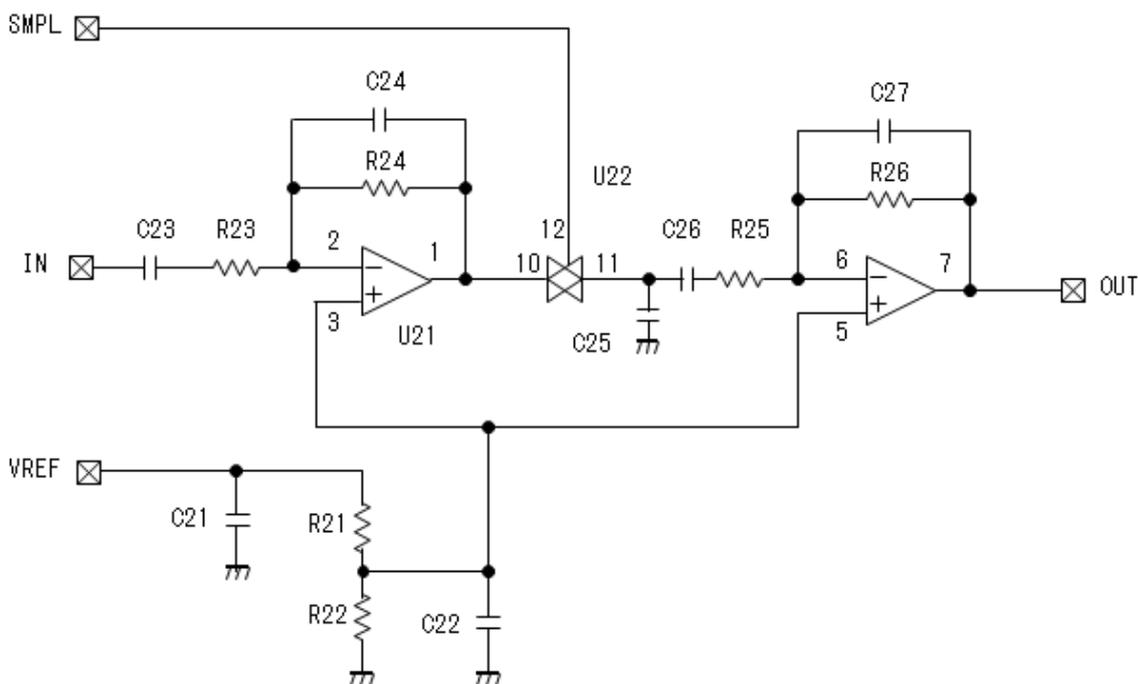
Figure 3-5 Example of Intermittent-Drive Pulse Wave Detector AFE Circuit
