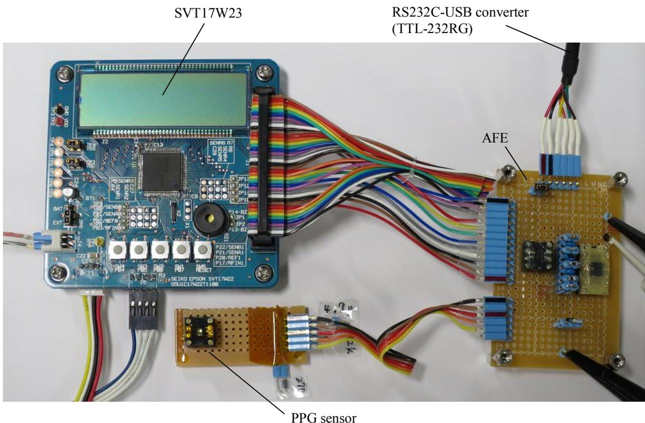
Figure 1-1 Evaluation System Used In Appendix A
