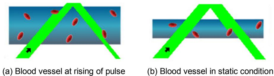
Figure 3-3 Reason for Light Intensity to Vary with Pulsation <sup>3)</sup>
