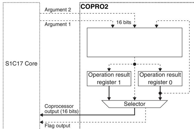
Figure 18.6.1 Data Path in Operation Result Read Mode
