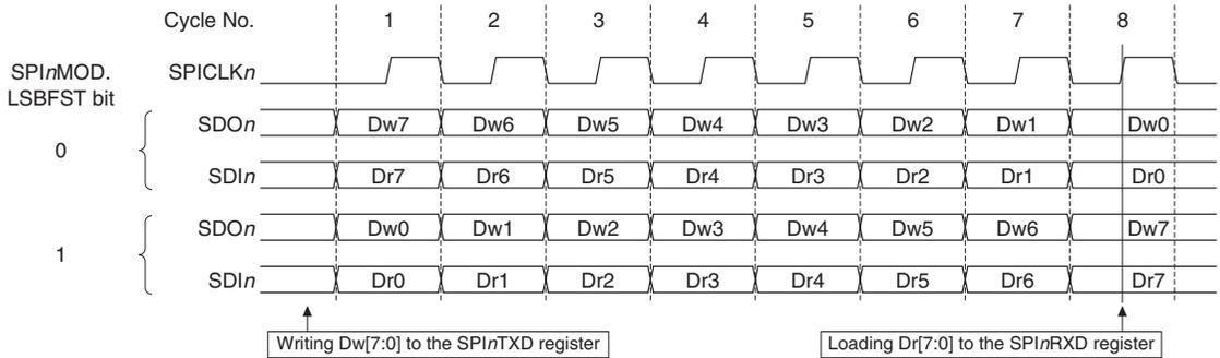
Figure 12.4.1 Data Format Selection Using the `SPInMOD.LSBFST` Bit
