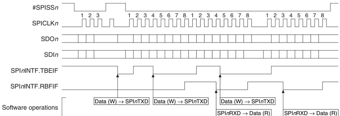
Figure 12.5.5.1 Example of Data Transfer Operations in Slave Mode ( $SPI_nMOD.CHLN[3:0]$  bits = 0x7)
