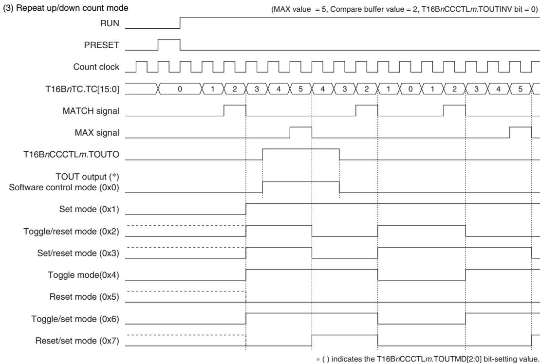
Figure 14.4.4.2 TOUT Output Waveform (T16BnCCCTLm.TOUTMT bit = 0)
