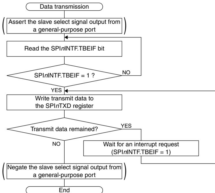
Figure 12.5.2.2 Data Transmission Flowchart in Master Mode
