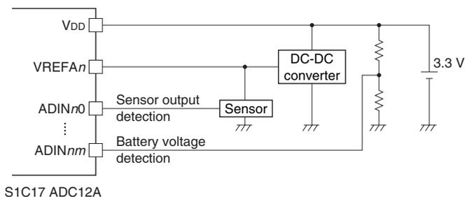
Figure 17.2.2.1 Connections between ADC12A and External Devices
