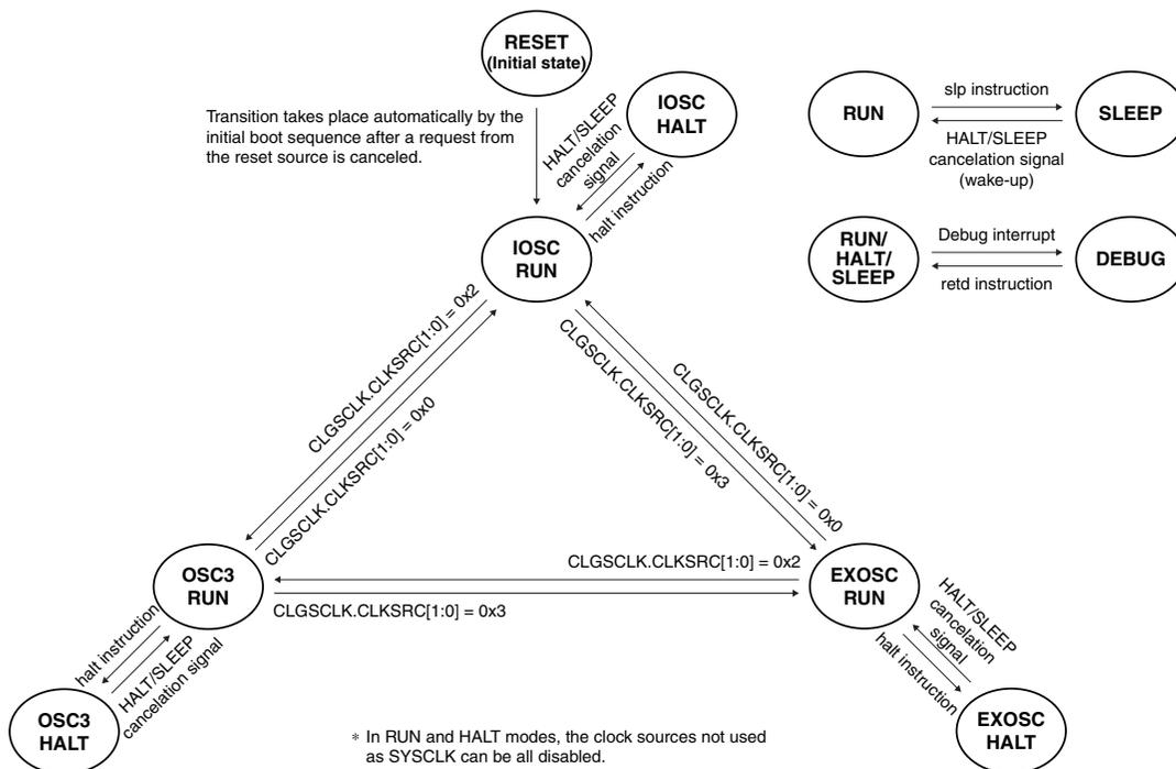
Figure 2.4.2.1 Operating Mode-to-Mode State Transition Diagram
