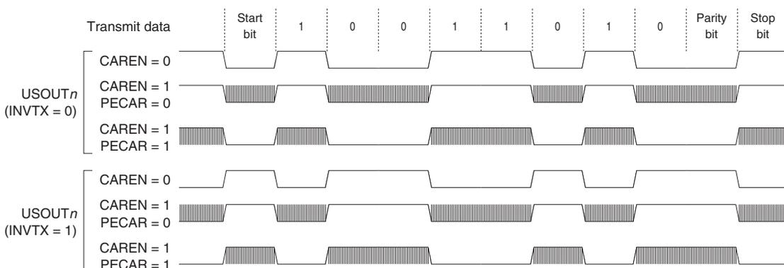
Figure 11.5.5.1 Carrier Modulation Waveform (UAnMOD.CHLN = 1, UAnMOD.STPB = 0, UAnMOD.PREN = 1)
