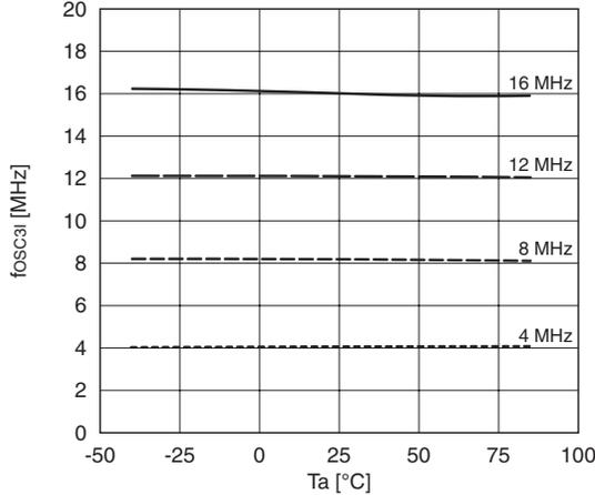
**EXOSC external clock input characteristics**
