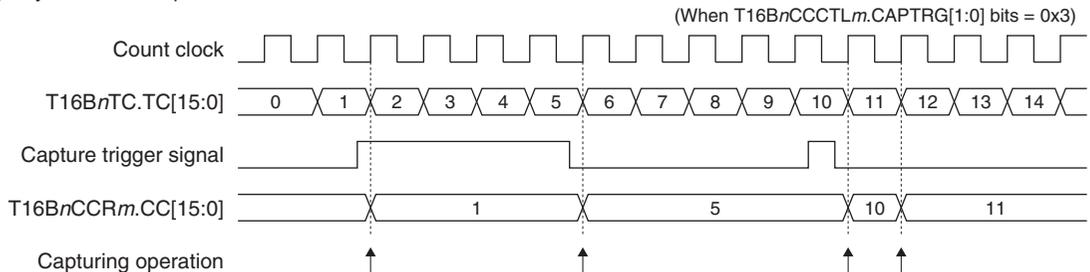
Figure 14.4.3.4 Synchronous Capture Mode/Asynchronous Capture Mode
