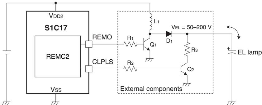
Figure 15.6.1 Example of EL Lamp Drive Circuit
