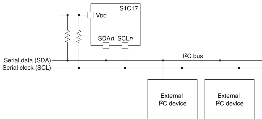
Figure 13.2.2.1 Connections between I<sup>2</sup>C and External I<sup>2</sup>C Devices
