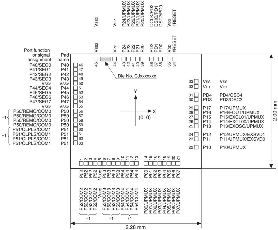
Figure 1.3.2.1 S1C17M12 Pad Configuration Diagram (Chip)
