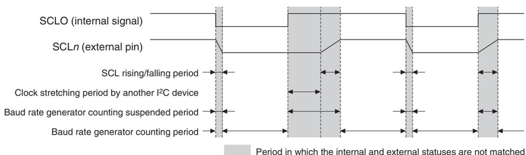
Figure 13.3.3.1 Baud Rate Generator Output Clock and SCL<sub>n</sub> Output Waveform
