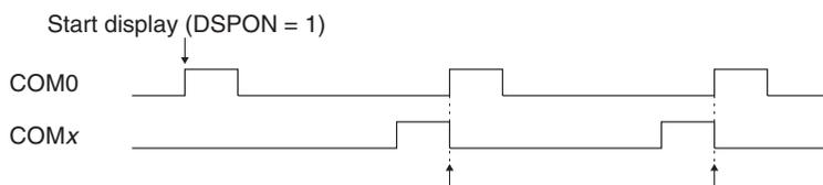
Figure 16.5.1 COM0 Lighting Interrupt Timings (Anode Common)
