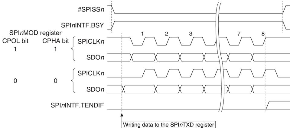
Figure 12.6.1 SPI<sub>n</sub>INTF.BSY and SPI<sub>n</sub>INTF.TENDIF Bit Set Timings (when SPI<sub>n</sub>MOD.CHLN[3:0] bits = 0x7)
