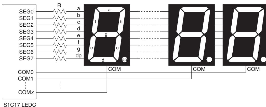
Figure 16.2.2.1 Connections between LEDC and Seven-Segment LED Modules
