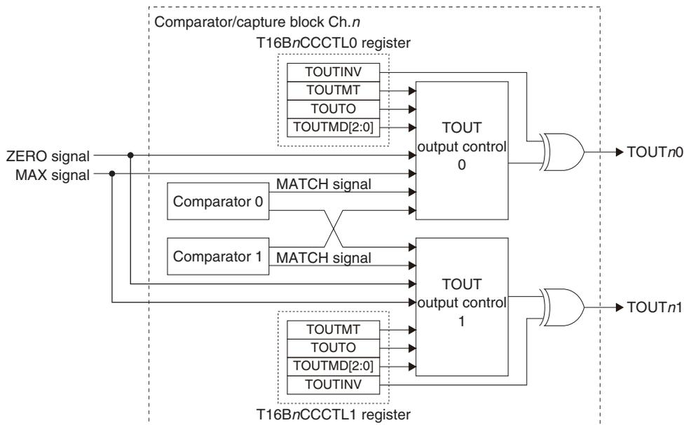
Figure 14.4.4.1 TOUT Output Circuits (Circuits 0 and 1)
