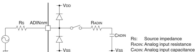
Figure 17.3.2.1 Equivalent Circuit of Analog Input Portion
