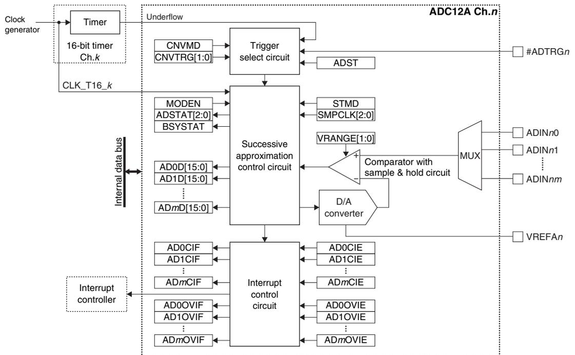
Figure 17.1.1 ADC12A Configuration
