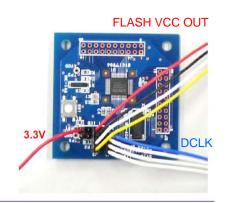
Please get power supply from emulator or stabilized power source for the evaluation board. (The red 3 Volt terminal in the back-right corner is used in this case.)
