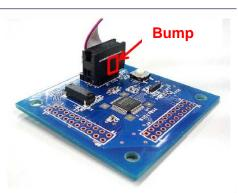
7.1.8 Please connect the emulator and the evaluation board with the PC. Check if both green and red LEDs are on. If those do not turn on, please check the connection.
