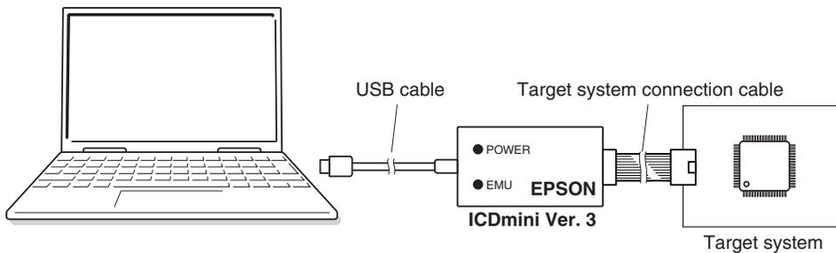
Figure 2.7.1.1 Example of Debugging System Using ICDmini3
