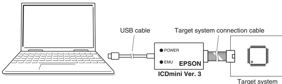
Figure B.2.1 Example of Debugging System Using ICDmini Ver. 3
