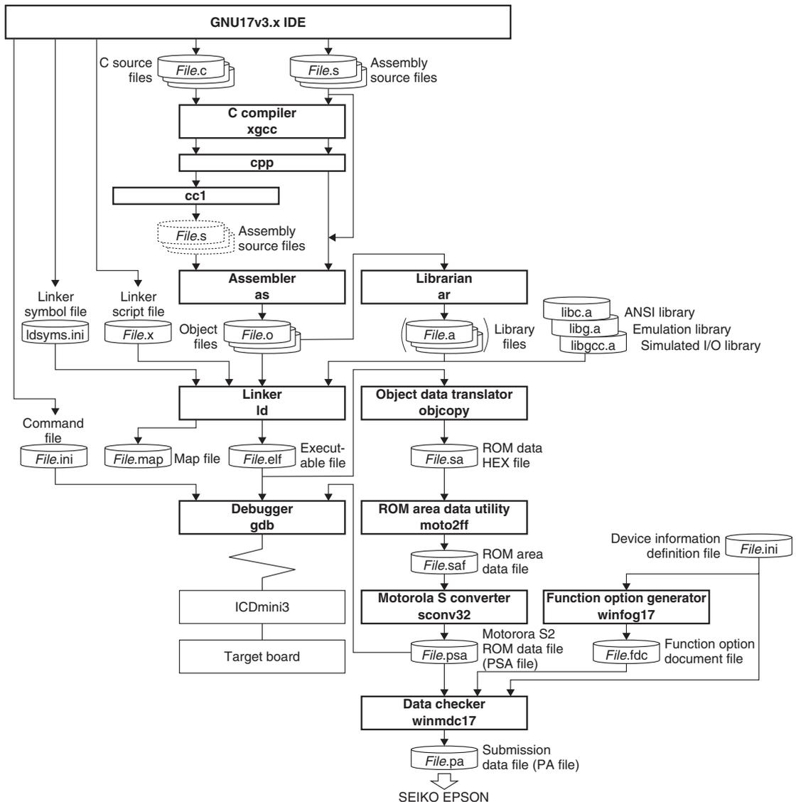
Figure 1.1.1 Configuration of Software Development Tools and Files
