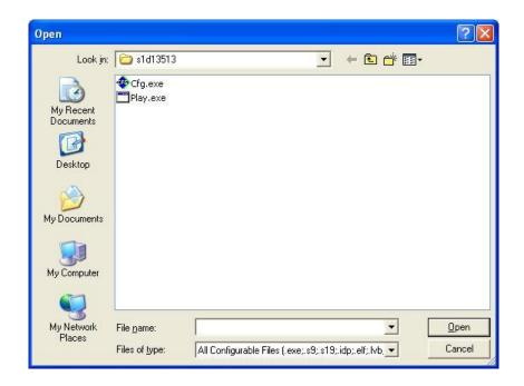
The Open option allows the 13513 CFG utility to read the configuration information from programs based on the API or HAL libraries. When 13513 CFG opens a file, it scans the file for an identification string, and if found reads the configuration information. This feature may be used to quickly arrive at a starting point for register configuration.
