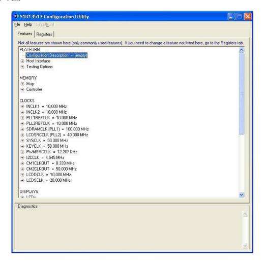
The Features Tab allows a specific S1D13513 configuration to be defined. All features are presented in a tree-control pane. The configuration is changed by selecting the desired setting for each feature. If the **panels.xml** and **cameras.xml** files are present in the same folder as the 13513 CFG utility, a number of predefined panel and predefined camera configurations are available.
