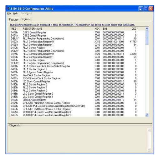
The Registers Tab allows viewing and editing of the S1D13513 register values. The registers are listed in the order in which they will be initialized by an application.
