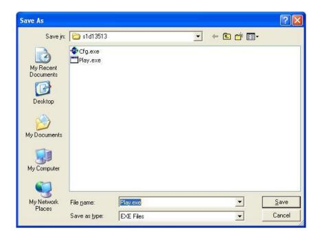
"Save As" is similar to Save, except the dialog permits renaming the file before it is saved. Using this technique, a user can configure a number of files differing only in configuration information and name.
