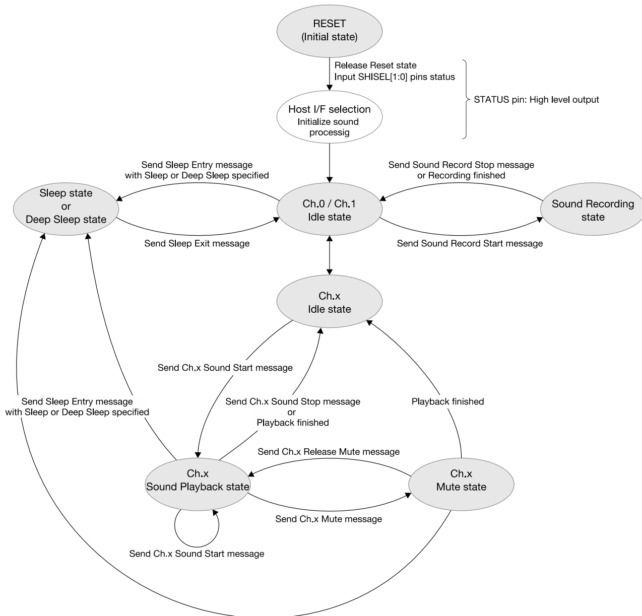
Figure 6.1 Internal Operating State Transition Diagram in Host Interface Mode
