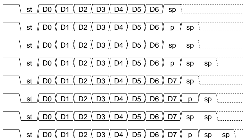
Figure 8.23 UART Data Format
