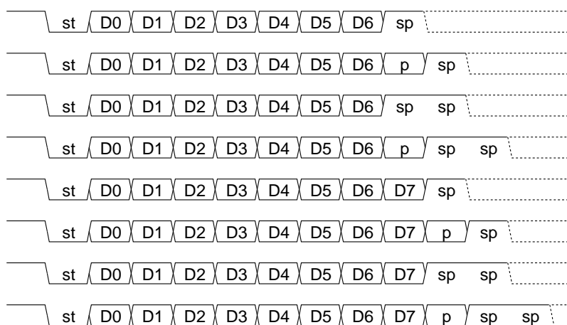
Figure 8.23 UART Data Format
