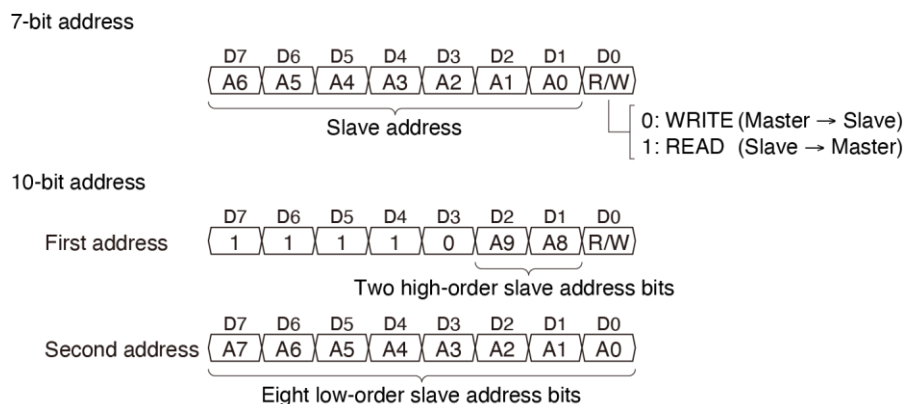
Figure 13.4.4.1 10-bit Address Configuration
